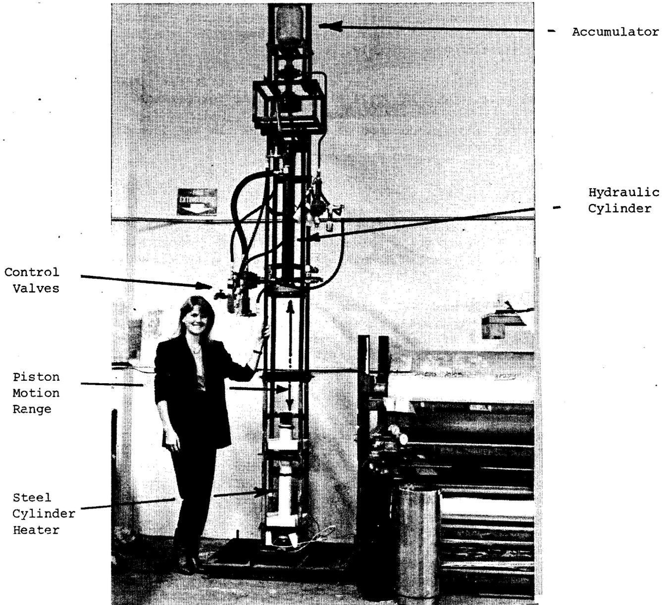
Figure 5-1. Hydraulic Shrink-fit Pin Insertion Apparatus for the Steel and DWAl 20® Hybrid Track Pin Production
