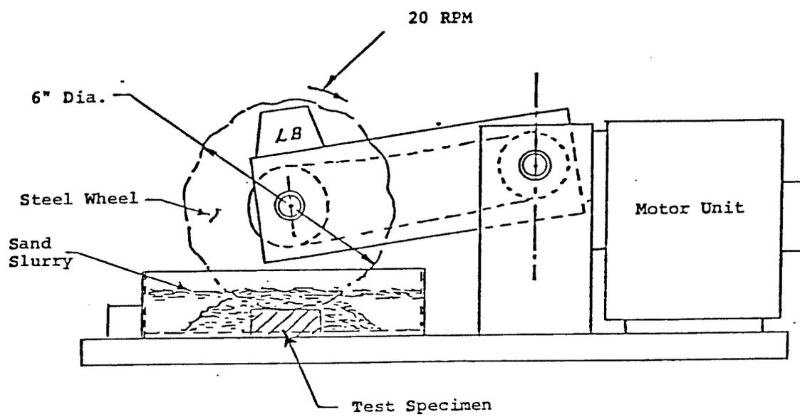
Figure 6-2. Schematic of Test Apparatus for Steel Wheel Abrasion Tests
