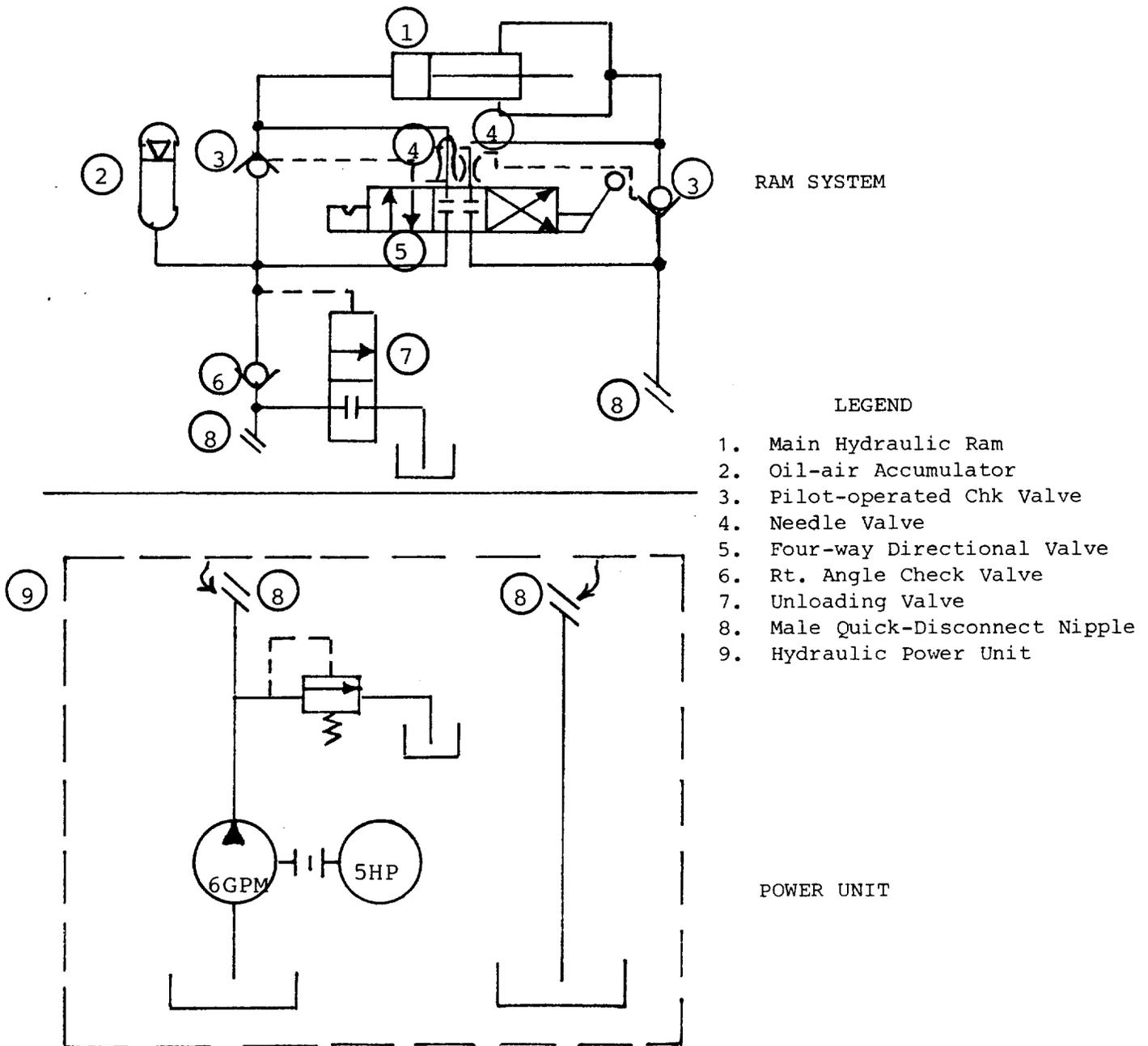
Figure 5-17. Schematic Diagram of Hydraulic-powered Pin Insertion Assembly Apparatus
