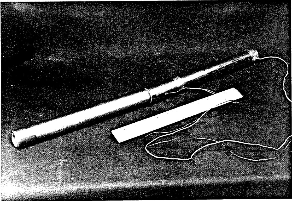
Figure 6-8. Post-Test Photograph of Instrumented Fatigue Test Track Pin
