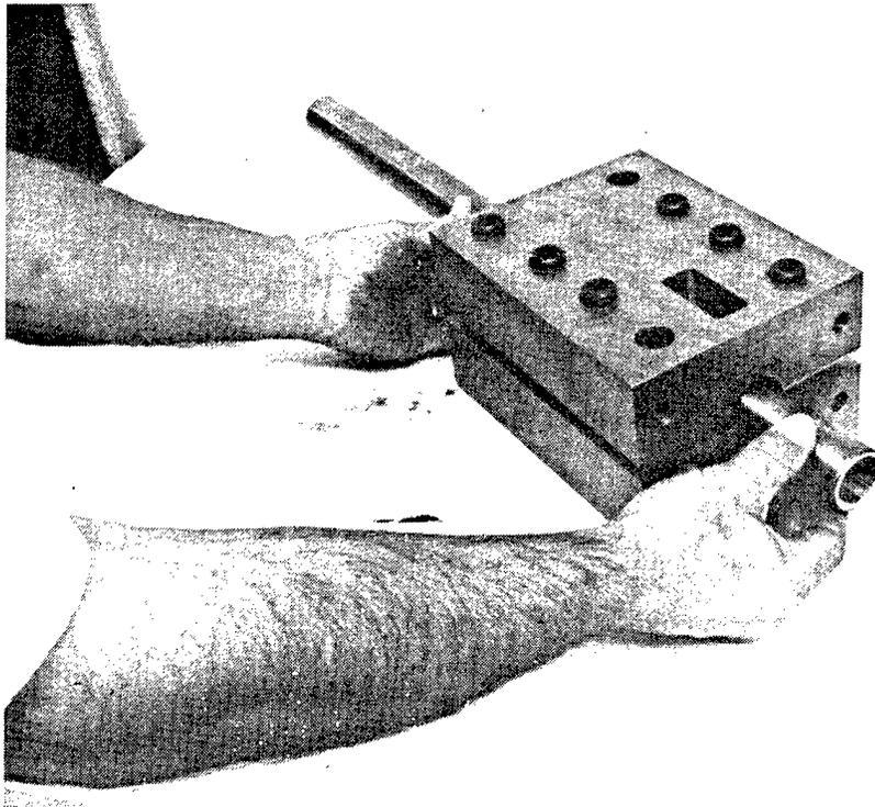
Figure 5-21. Installing DWAL 20<sup>®</sup> and Steel Track Pin into Pin-end Crimp-forming Tool
