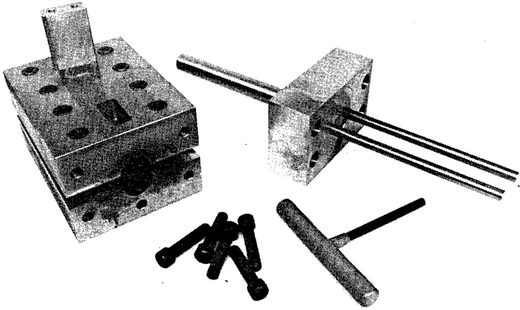
Figure 5-20. Component Parts of Pin-end Crimp-forming Tool
