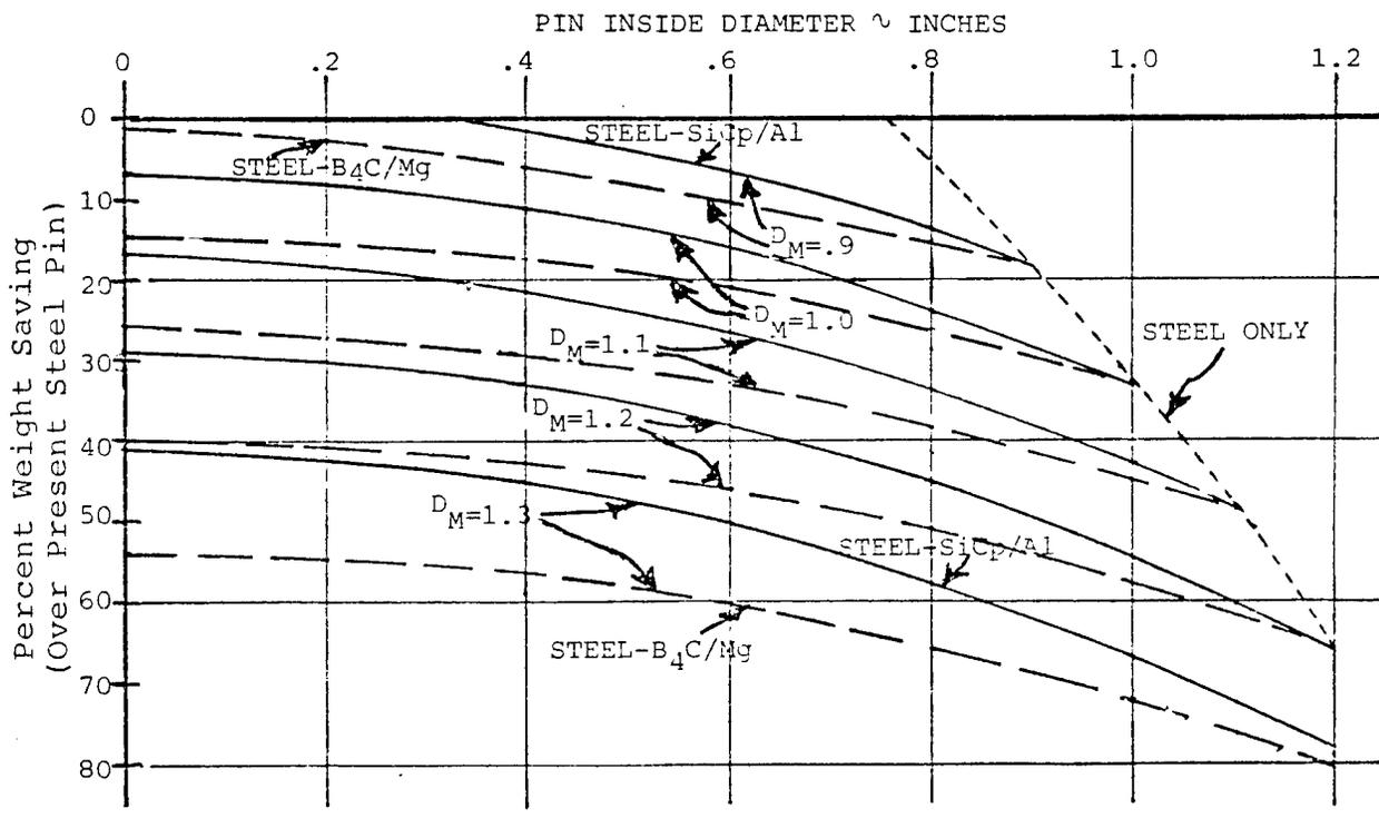
Figure 5-3. Overview of Candidate Pin Configurations, Comparing Potential Weight Savings
