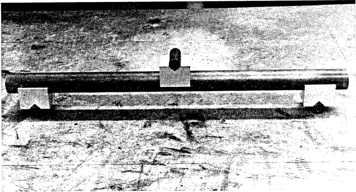
Figure 6-5. Sample Track Pin Installed on Test Pillow Blocks with a Third Pillow Block Centered on Top
