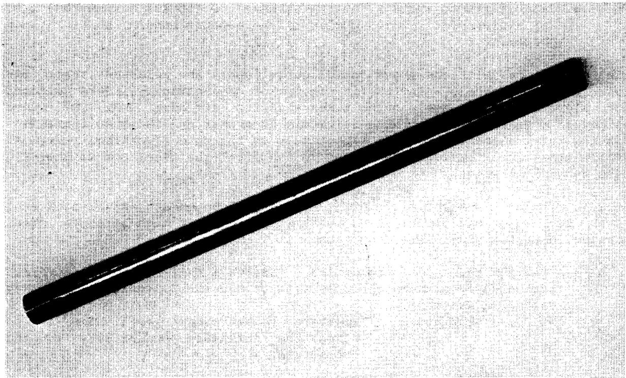
Figure 5-2. Lightweight Track Pin Constructed of DWAl 20<sup>®</sup> Metal Matrix Composite Encased in a Steel Jacket
