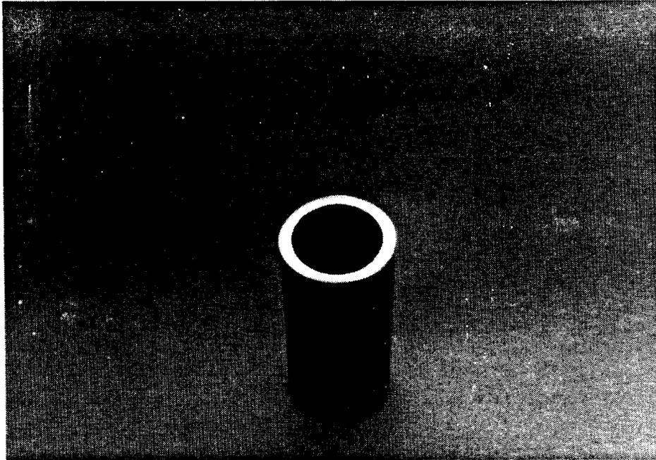
Subsize Hybrid Pin Section, 4130 Steel Jacket Enclosing DWAl 20<sup>®</sup> Tubular Sleeve, 20v/o SiCp/6061
