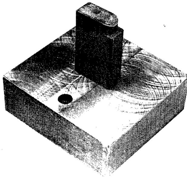
Figure 5-26. Pin-end Crimp-former Punch Installed on Pressure Plate to Prevent Cocking During Pin-end Shaping Operation
