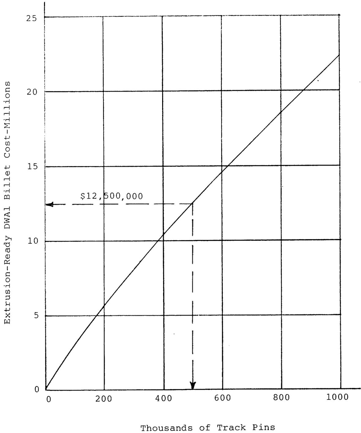
Figure 7-1. Cost of DWAL 20<sup>®</sup> Billets Required for Production of the Hybrid Lightweight MBT Track Pin
