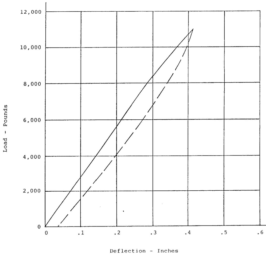
Figure 6-4. Results of Static Testing a Final Hybrid Lightweight Track Pin
