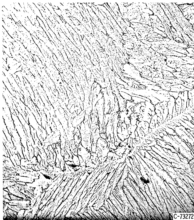
Figure 4. - Microstructure of sample containing 76.2 atomic percent vanadium. Primary phase, V_3Ga (white); secondary phase, V-Ga solution. Etchant, 4H_2O-3HNO_3-1HF ; X250.
