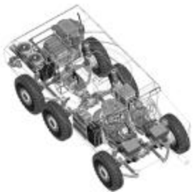
Combat Hybrid Power System (CHPS) Notional Concept Vehicle
