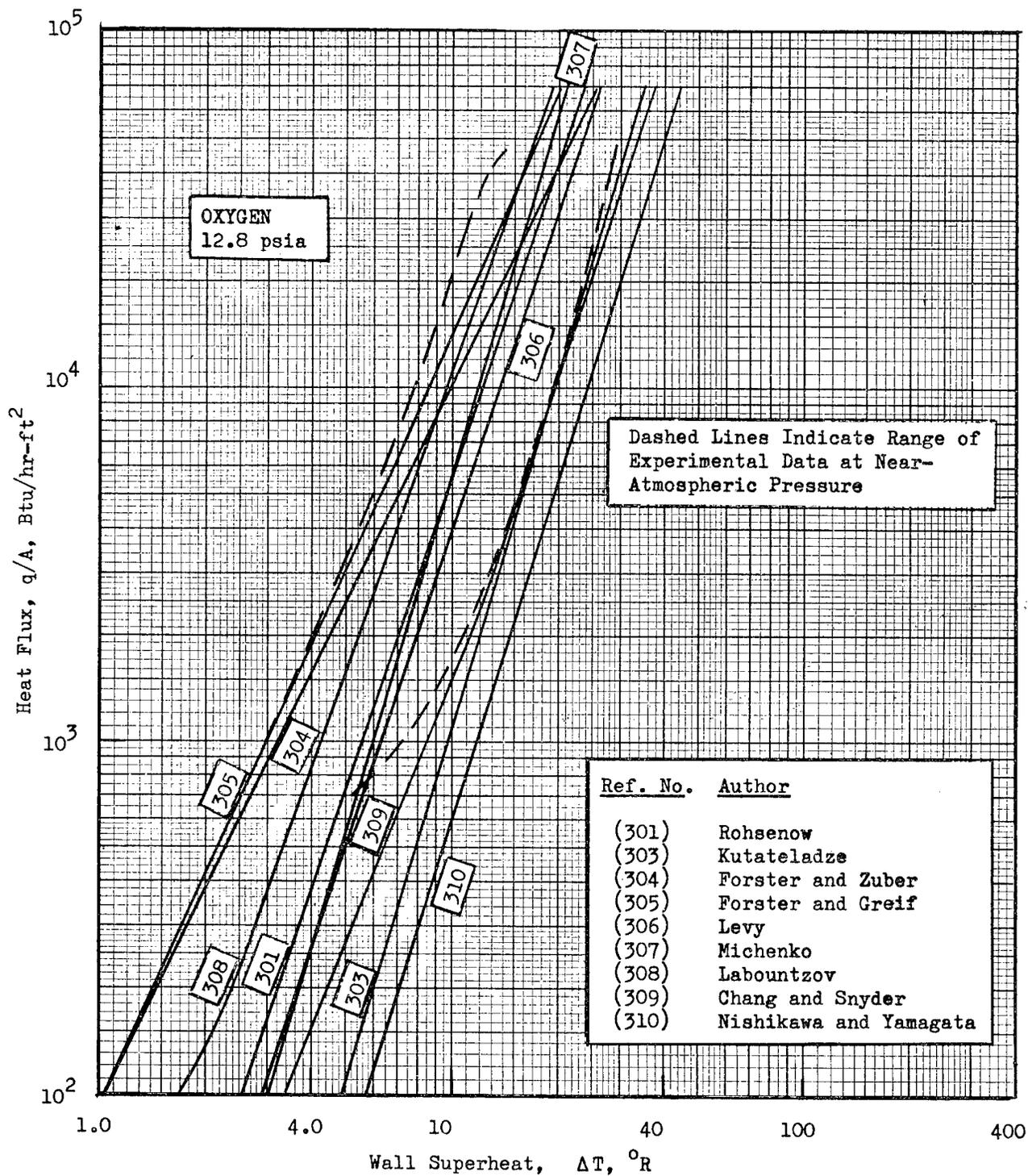
FIG. 6 POOL NUCLEATE BOILING OF OXYGEN AT 12.8 PSIA
