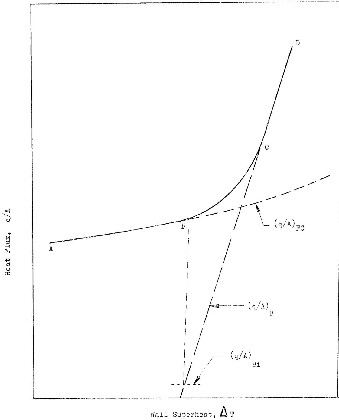
FIG. 21 TYPICAL FORCED CONVECTION SUBCOOLED NUCLEATE BOILING CURVE
