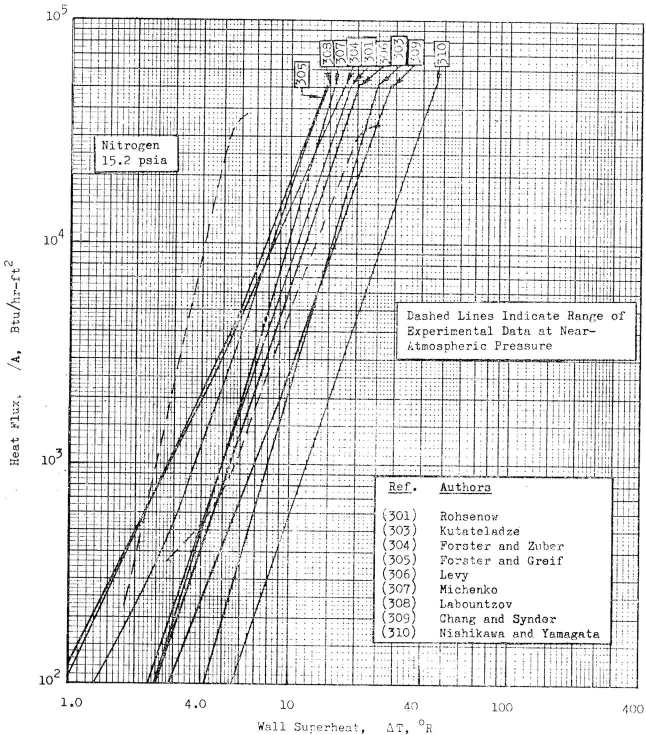
FIG. 5 POOL NUCLEATE BOILING OF NITROGEN AT 15.2 PSIA
