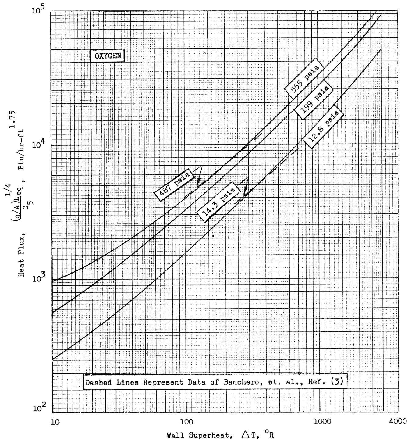
FIG. 20 STABLE POOL FILM BOILING OF OXYGEN
