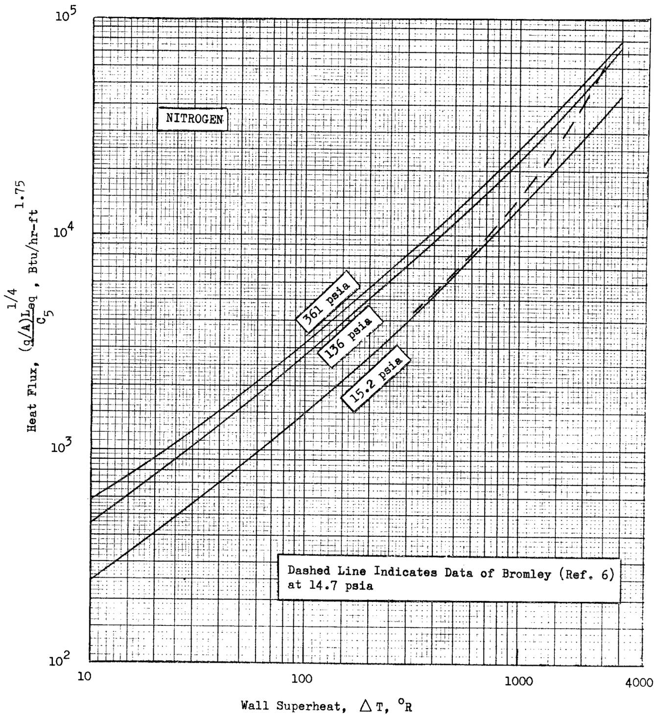
FIG. 19 STABLE POOL FILM BOILING OF NITROGEN
