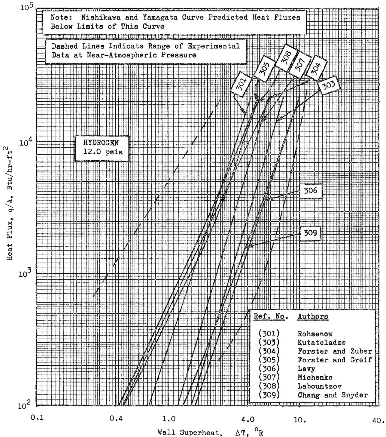
FIG. 4 POOL NUCLEATE BOILING OF HYDROGEN AT 12.0 PSIA
