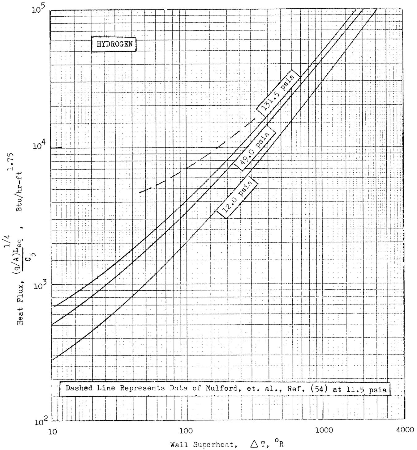
FIG. 18 STABLE POOL FILM BOILING OF HYDROGEN
