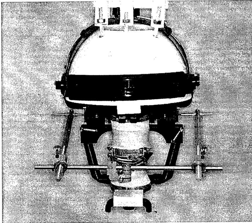
Figure 4: The maxillary and mandibular pantographic reference plates, Stuart reference pantographic reference plates.
