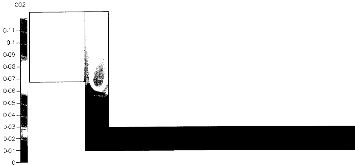
Figure 86. Simulation 6, plan view (D-D) depicting CO 2 (mass fraction) distribution throughout the structure.
