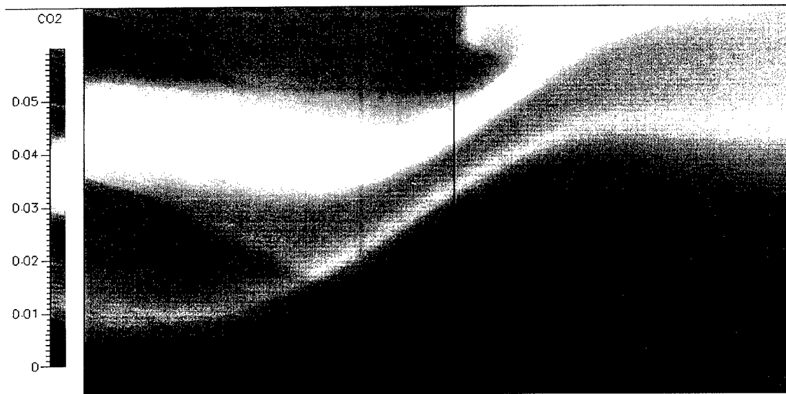
Figure 76. Simulation 6, partial elevation view (A-A) of CO 2 gas (mass fraction) propagation at the centerline of the longitudinal passageway in the vicinity of the watertight door.
