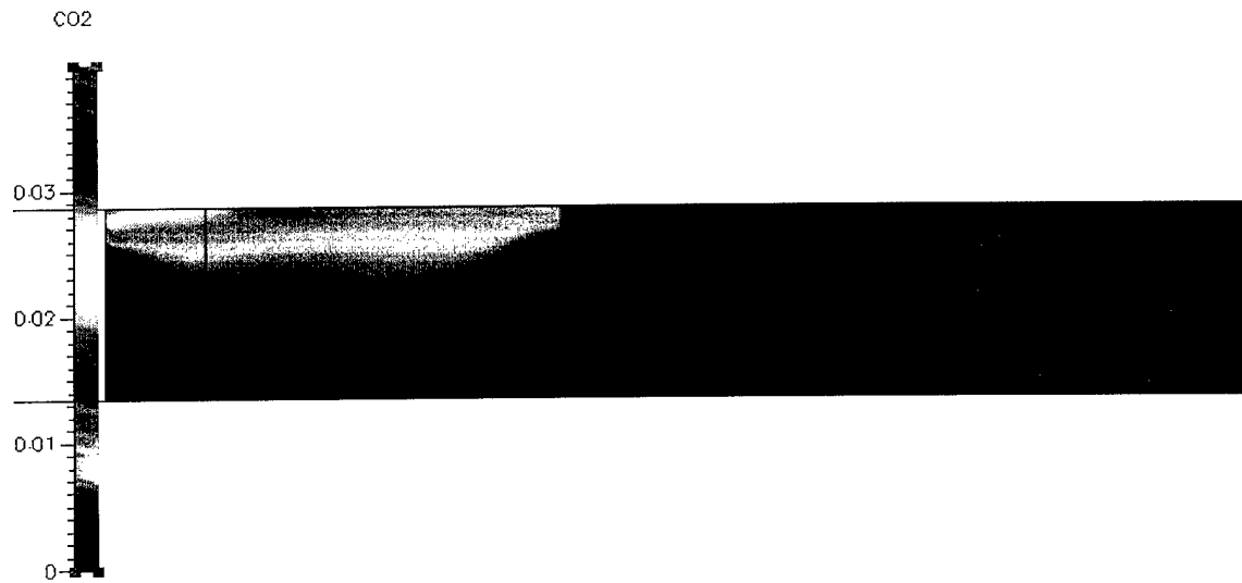
Figure 90. Simulation 7, elevation view (A-A) of CO 2 gas (mass fraction) propagation at the centerline of the longitudinal passageway.
