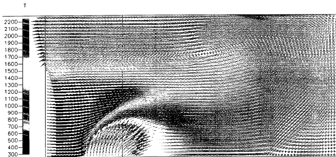
Figure 13. Simulation 1, partial elevation view (B-B) depicting temperature (K) distribution and fluid circulation pattern along the centerline of the transverse passageway on the port side of the structure.
