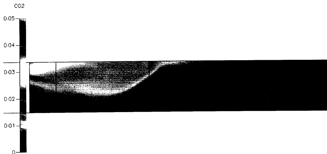
Figure 38. Simulation 3, elevation view (A-A) of CO 2 gas (mass fraction) propagation at the centerline of the longitudinal passageway.
