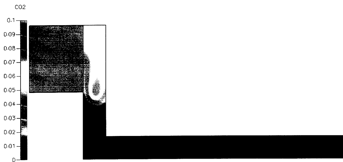
Figure 21. Simulation 1, plan view (D-D) depicting CO 2 (mass fraction) distribution throughout the structure.
