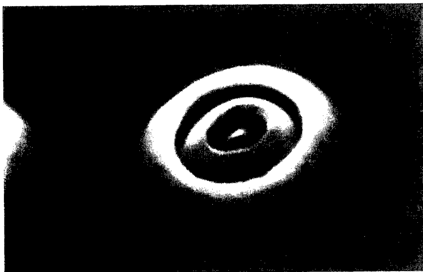
Figure 28. SEM micrograph of a single-tip gated field emitter with a 0.4\ \mu\text{m} thick Cr gate (inner rim). The gate diameter is 1.4\ \mu\text{m} .
