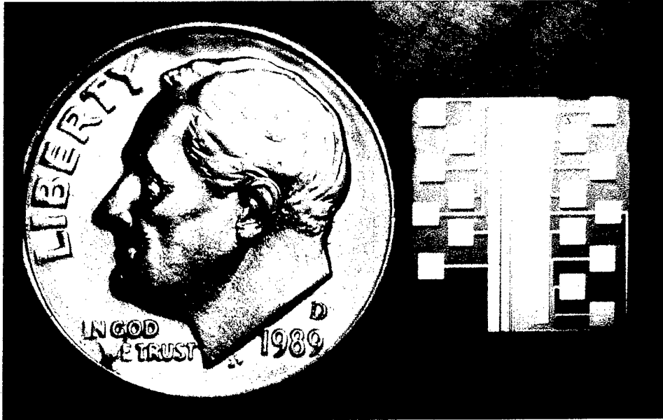
Figure 5. A glass submount containing many electrodes was used to direct an electric field across an individual KTP waveguide for electro-optic control.
