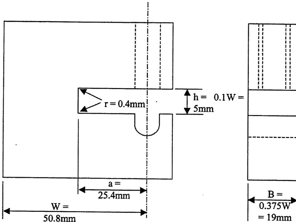
Figure 7. Configuration of modified bolt-loaded compact specimen.
