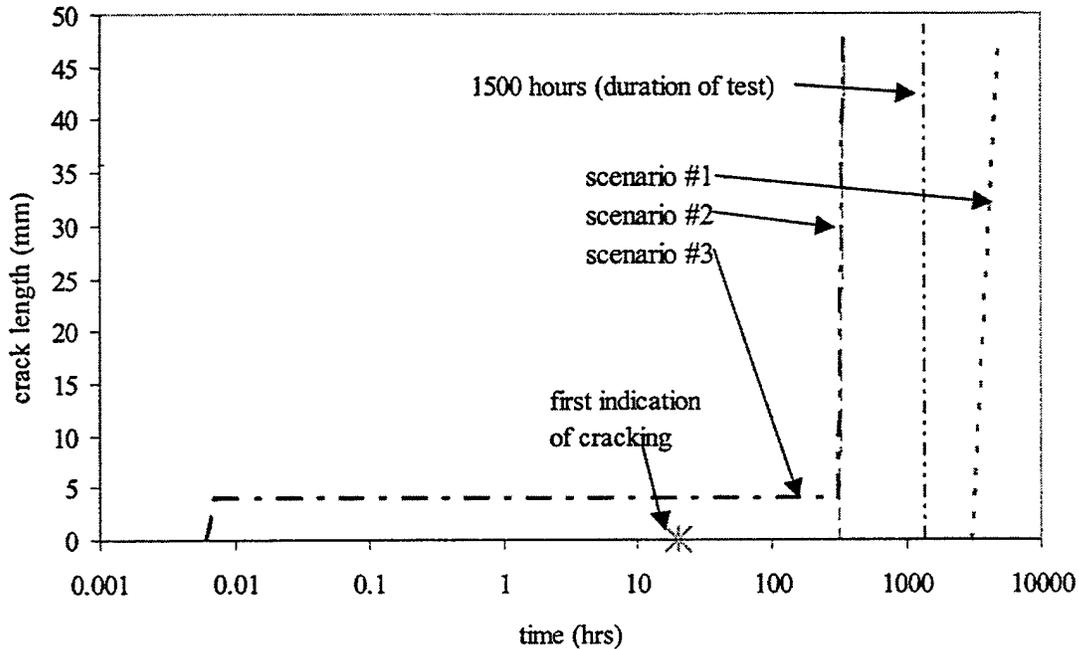
Figure 10. Modeling of several hydrogen cracking scenarios.
