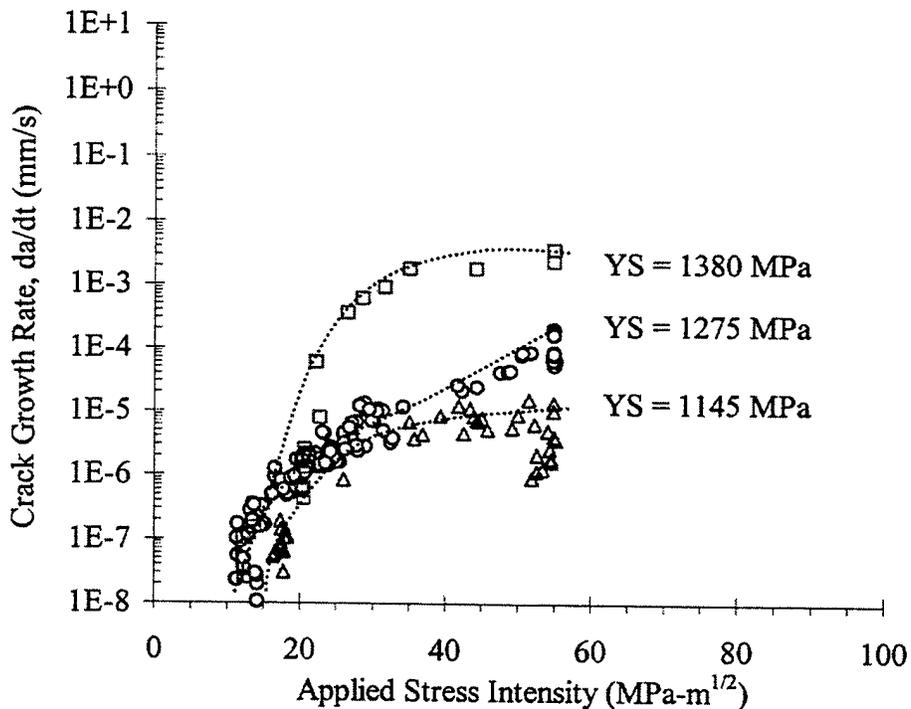
Figure 2.  $da/dt$  versus  $\Delta K$  in 50% H<sub>2</sub>SO<sub>4</sub>/50% H<sub>3</sub>PO<sub>4</sub> acid for ASTM A723 steel at three different strength levels.
