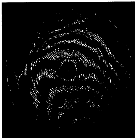
Figure 4.10 Interferogram from the video camera of the phase-shifting interferometer. Note the uniform intensity of the fringes over the outer half of the pupil.
