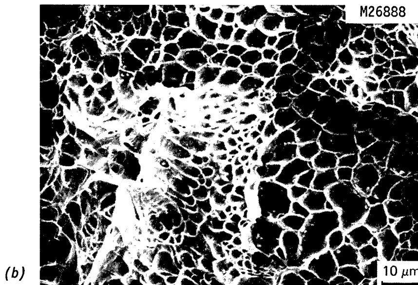
Fig. 7. SEM micrographs of \text{ZrO}_2 half of \text{ZrO}_2 -Fe specimen tested at 400^\circ\text{C} : (a) overall appearance, and (b) fracture appearance in Cu plating.
