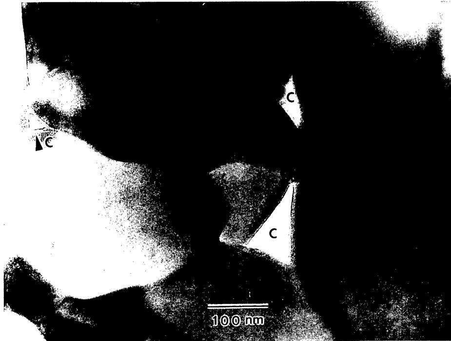
Fig. 5. TEM micrograph from sample after tensile creep at 1200°C showing cavities produced at triple grain junctions as a result of deformation.
