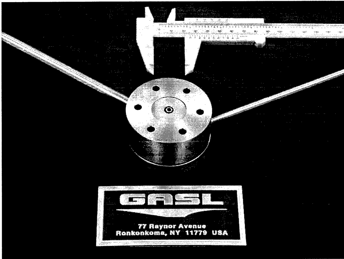
Figure 14 Photo of assembled N_2O and C_3H_8 modular injectors. The center orifice is the C_3H_8 injector concentric with the sintered mesh orifice. This annular region is designed to allow 75% of the total N_2O flow to pass through.
