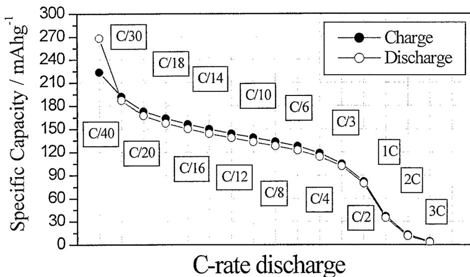
Figure 5. Capacity versus discharge rate of the Li / P(EO)<sub>20</sub>LiCF<sub>3</sub>SO<sub>3</sub> +10 w/o neutral Al<sub>2</sub>O<sub>3</sub> / LiMn<sub>3</sub>O<sub>6</sub> polymer battery at 105°C. Charge rate: C/10. Voltage window: 3.7 V – 1.5 V. Cathode source: US Army, Fort Monmouth.
