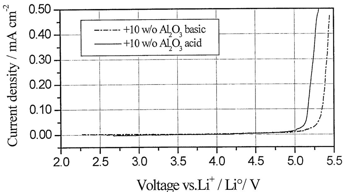
Figure 1. Current-voltage curve of a stainless-steel electrode in  $\text{P(EO)}_{20}\text{LiCF}_3\text{SO}_3$  +10 w/o  $\text{Al}_2\text{O}_3$  polymer electrolyte cells. Counter and reference electrode: Li.  $T=95^\circ\text{C}$ . Scan rate  $0.2\text{mV/s}$ .
