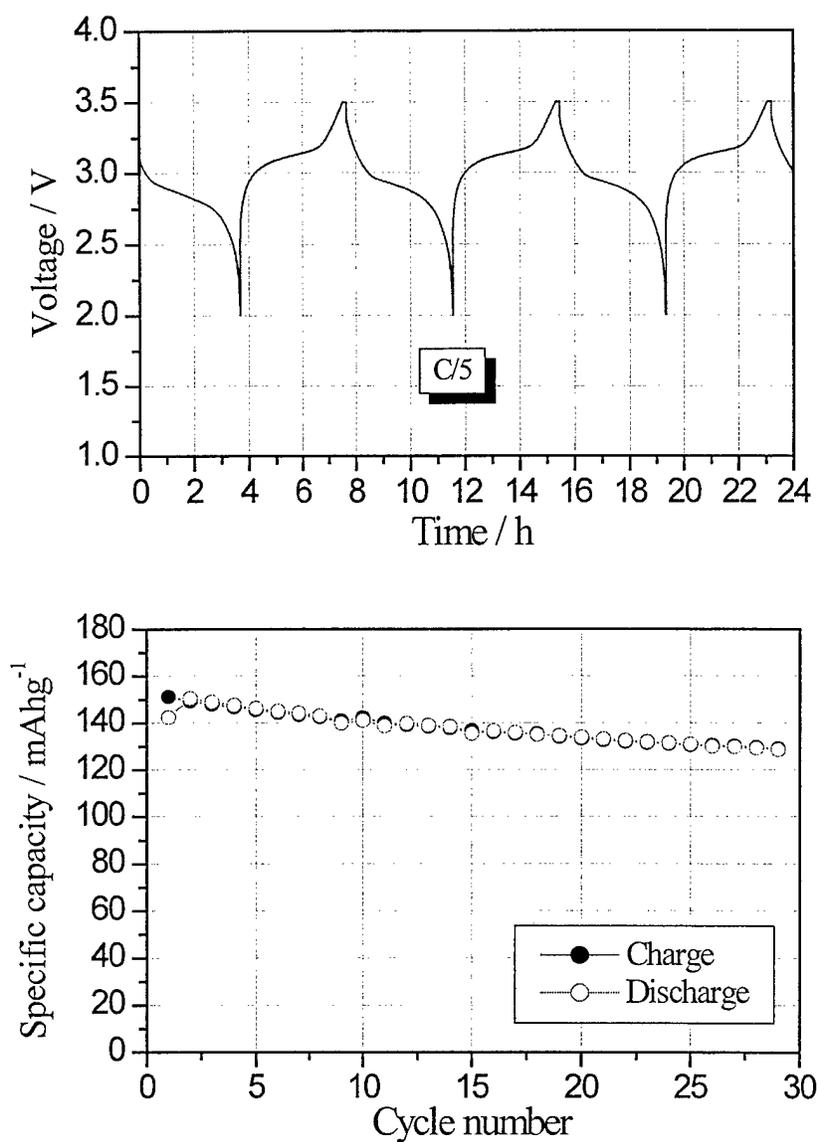
Figure 8. Voltage profiles (upper panel) and capacity delivery (lower panel) of the Li / P(EO)<sub>20</sub>LiCF<sub>3</sub>SO<sub>3</sub> +10 w/o neutral Al<sub>2</sub>O<sub>3</sub> / LiMn<sub>3</sub>O<sub>6</sub> polymer battery cycled 70 °C. Charge-discharge rate: C/5. Voltage window: 3.5 V – 2 V. Cathode composition: 80 wt% LiMn<sub>3</sub>O<sub>6</sub>, 10 wt% PEO (M.W. 4 000 000), 10 wt% Super P. Current density: 71 μAcm<sup>-2</sup>. T = 70°C. Cathode source: Chunco Denki Kogyo Co. LTD.
