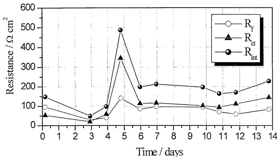
Figure 3. Time evolution of the resistance parameters of the  $\text{Li/P(EO)}_{20}\text{LiCF}_3\text{SO}_3 + 10 \text{ w/o Al}_2\text{O}_3 \text{ acid /Li}$  cell stored under open circuit conditions at  $95^\circ\text{C}$ . The values of the total interfacial resistance,  $R_i$ , and of its components, i.e. the passivation film resistance,  $R_f$  and the charge transfer resistance,  $R_{ct}$ , have been evaluated by fitting impedance experimental results.
