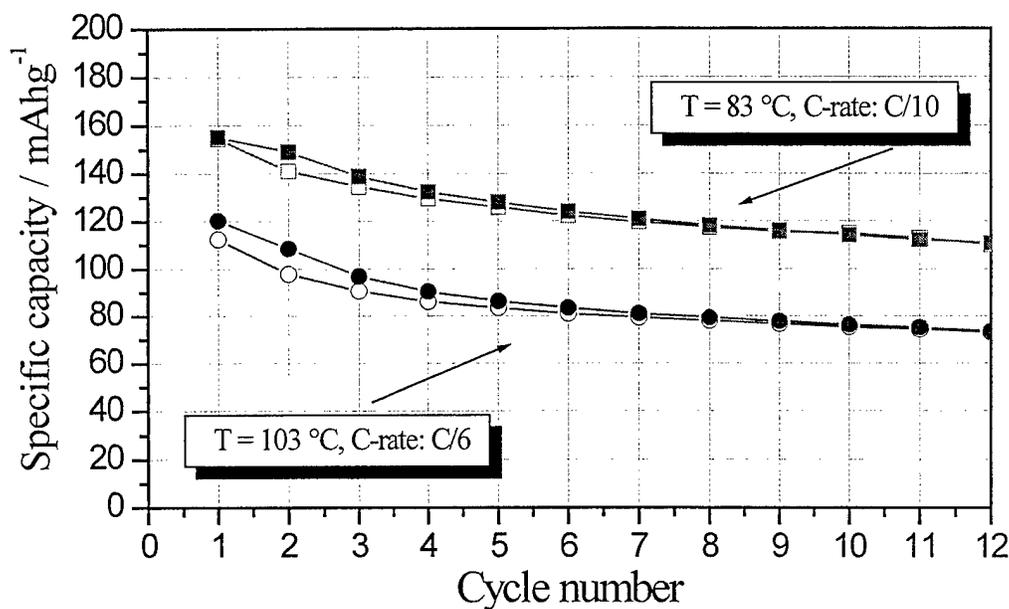
Figure 7. Comparison between the capacity delivery (lower panel) of the Li /  $\text{P}(\text{EO})_{20}\text{LiCF}_3\text{SO}_3 + 10 \text{ w/o neutral Al}_2\text{O}_3 / \text{LiMn}_3\text{O}_6$  polymer battery cycled at  $83^\circ\text{C}$  and at  $103^\circ\text{C}$ . Charge-discharge rate: C/10. Voltage window: 3.7 V – 1.5 V. Cathode source: US Army, Fort Monmouth.
