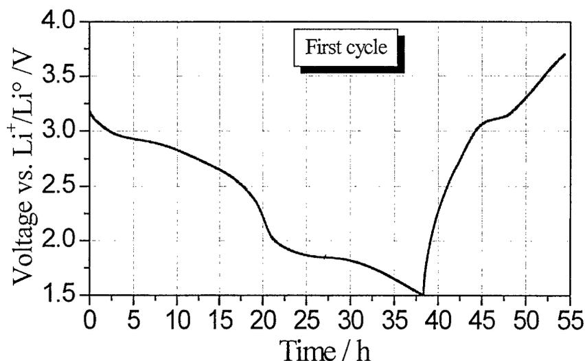
Figure 4. Voltage versus time profile of a low- rate, galvanostatic discharge of the Li / P(EO)<sub>20</sub>LiCF<sub>3</sub>SO<sub>3</sub> +10 w/o neutral Al<sub>2</sub>O<sub>3</sub> / LiMn<sub>3</sub>O<sub>6</sub> polymer battery at 105°C and in the 3.7 V – 1.5 V voltage window. The discharge curve is followed by a medium rate charge.
