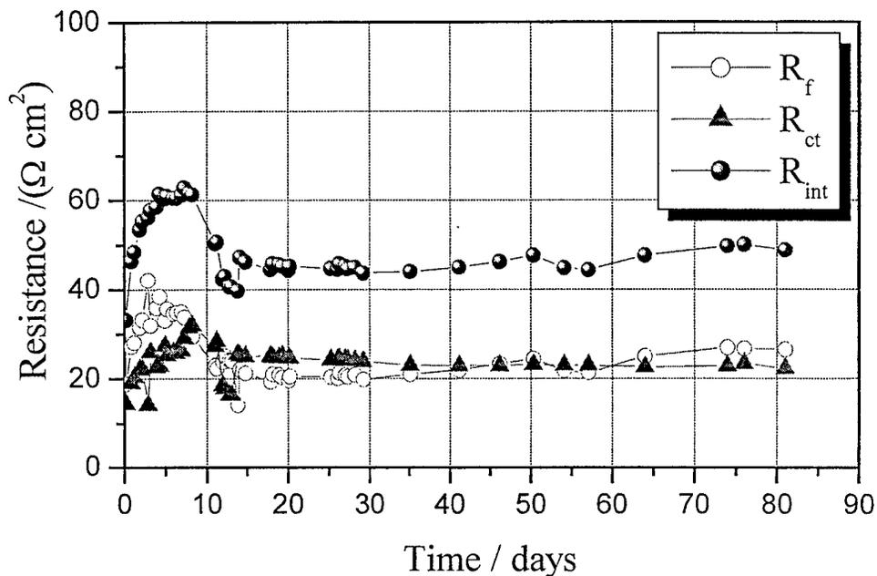
Figure 2. Time evolution of the resistance parameters of the Li/P(EO)<sub>20</sub>LiCF<sub>3</sub>SO<sub>3</sub> +10 w/o Al<sub>2</sub>O<sub>3</sub> neutral /Li cell stored under open circuit conditions at 95 °C. The values of the total interfacial resistance,  $R_i$ , and of its components, i.e. the passivation film resistance,  $R_f$  and the charge transfer resistance,  $R_{ct}$ , have been evaluated by fitting the impedance experimental results .
