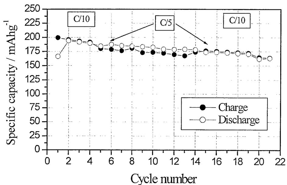
Figure 9 Capacity delivery upon cycling of the Li / P(EO)<sub>20</sub>LiCF<sub>3</sub>SO<sub>3</sub> +10 w/o neutral Al<sub>2</sub>O<sub>3</sub> / LiMn<sub>3</sub>O<sub>6</sub> polymer battery at 70°C. Charge-discharge rate: C/10. Voltage window: 3.5 V – 2.0 V. The discharge was run in the galvanostatic mode and the charge in the mixed galvanostatic – potentiostatic mode.
