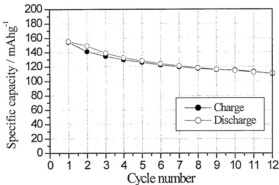
Figure 6. Capacity delivery upon cycling of the Li /  $\text{P}(\text{EO})_{20}\text{LiCF}_3\text{SO}_3 + 10 \text{ w/o neutral Al}_2\text{O}_3 / \text{LiMn}_3\text{O}_6$  polymer battery at  $105^\circ\text{C}$ . Charge-discharge rate: C/10. Voltage window: 3.7 V – 1.5 V. The discharge was run in the galvanostatic mode and the charge in the mixed galvanostatic – potentiostatic mode. Cathode source: US Army, Fort Monmouth.
