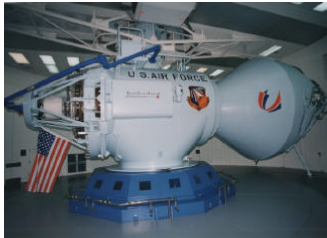
Figure 5. Dynamic Environment Simulator (DES) Centrifuge
