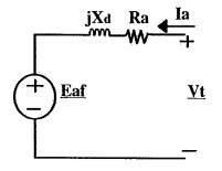
Figure 5-12: Equivalent circuit diagram for synchronous motor.
