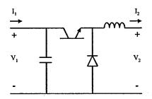
Figure 8-6: Buck converter simplified circuit.
