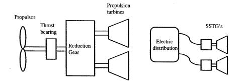
Figure 1-1: Mechanical drive schematic.
