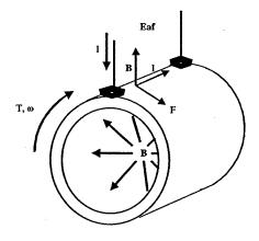
Figure 7-1: Single turn homopolar motor.
