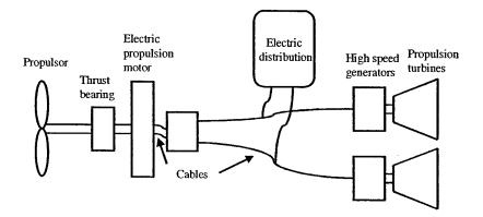
Figure 1-2: Electric drive schematic
