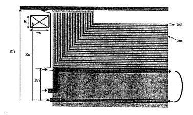
Figure 7-4: Cross section of 1/4 of hybrid HPM showing water cooling in inner drum and wetted C02 cooling on outer side of drum turns. Rri - inner drum radius, trot - drum thickness, tins - spacing between drums, Rfs - inner radius of flux shield, Rc - Coil mean radius, tc/wc - coil thickness and width.
