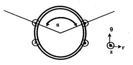
Figure 5-4: Short-pitched coils showing azimuthal angle extent,  $\alpha$ , of individual coil which is less than the full pitched angle of  $\pi$ .
