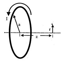
Figure 7-6: Circular current carrying coil
