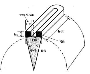
Figure 6-2: Superconducting pole head. Showing dimensions of field windings, minimum bend radius  $r_m$ , physical angle of extent  $\theta_{wf}$ , number of field windings  $N_{ft}$  and radius of field.
