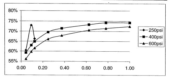
Using 600 psi saturated steam, a 2% reduction in efficiency is noted when the steam turbine is operated at 60% of its rated power. (Data derived from [20]).
