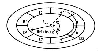
Figure 6-3: End turns required azimuthal traverse,  $l_{az}$ , belt to belt.
