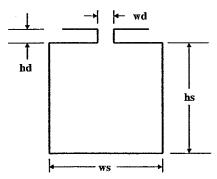
Figure 5-10: Single stator slot showing relative dimensions
