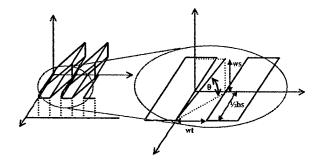
Figure 5-8: Armature winding departure path in slotted stator.
