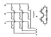
Figure 8-5: Matrix converter simplified circuit.[23]
