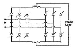
Figure 8-3: Cycloconverter simplified circuit.
