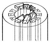
Figure 5-6: End turn winding arrangement. Showing angle of departure as windings move towards next slot opening and over adjacent windings.
