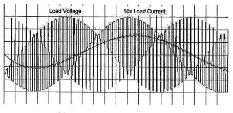
Matrix converter output waveform.
