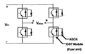
Figure 8-1: H-Bridge inverter used in 19 MW PWM AC/AC converter at the LBES
