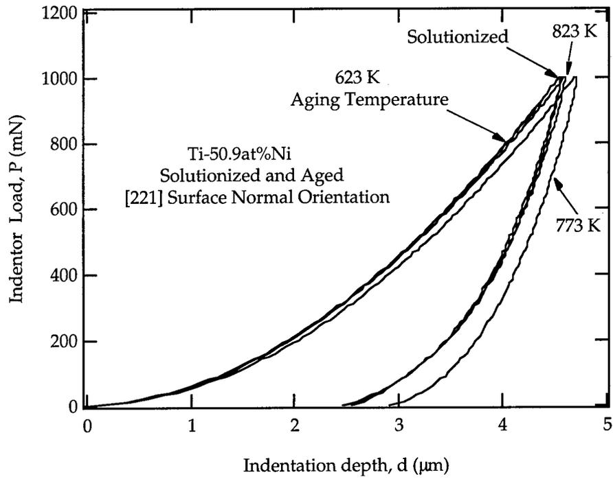
Figure 20: Loading curves for the [221] orientation.
