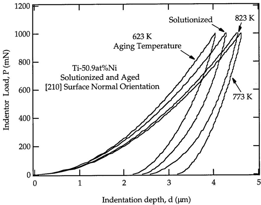
Figure 19: Loading curves for the [210] orientation.
