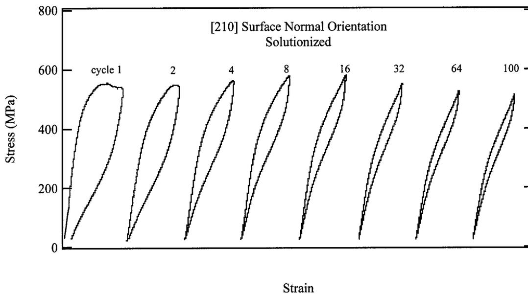
Figure 22: Compressive response of [210] oriented solutionized NiTi
