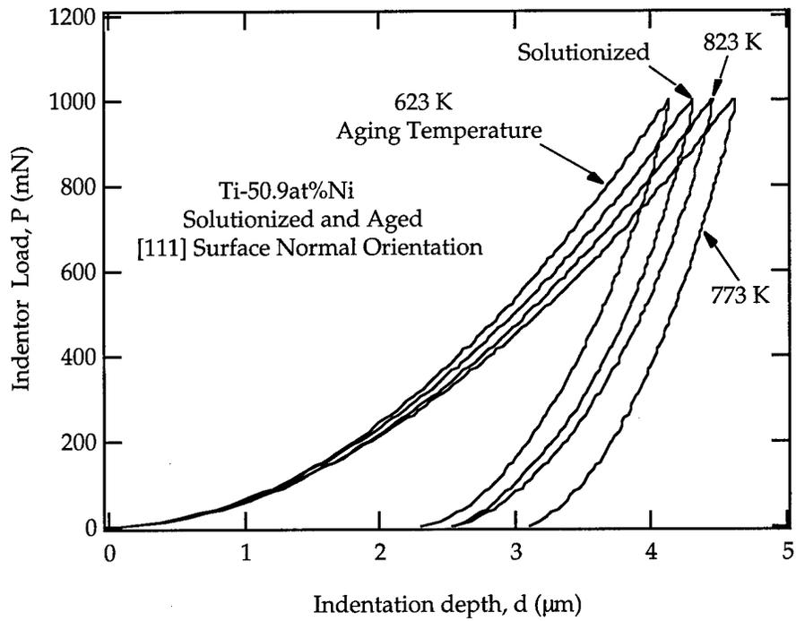
Figure 17: Loading curves for the [111] orientation.
