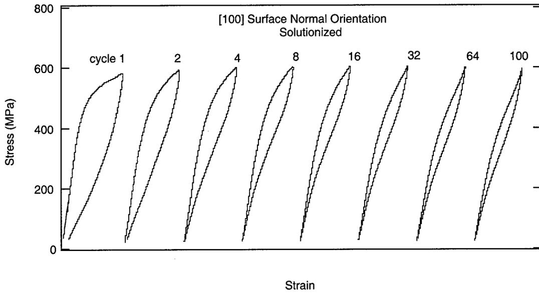
Figure 26: Compressive response of [100] oriented solutionized NiTi
