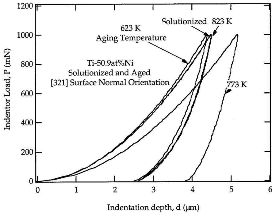
Figure 21: Loading curves for the [321] orientation.
