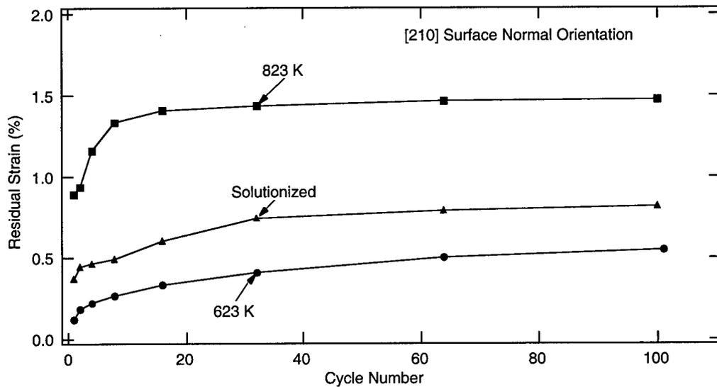
Figure 38: Residual strain accumulation for the [210] orientation
