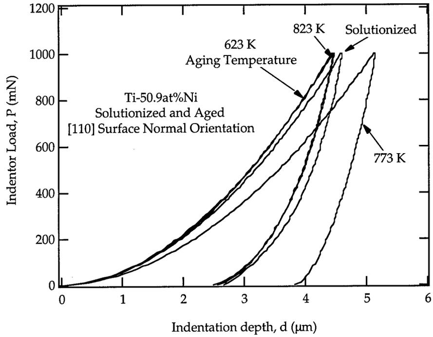
Figure 16: Loading curves for the [110] orientation.
