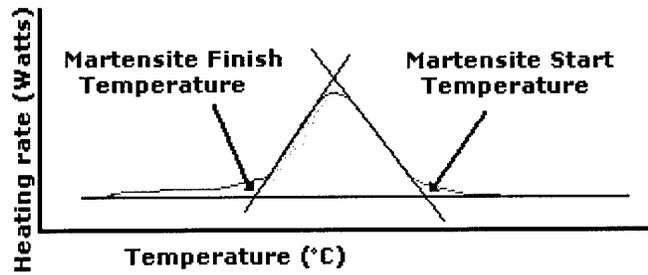
Figure 2: Determination of transition temperatures
