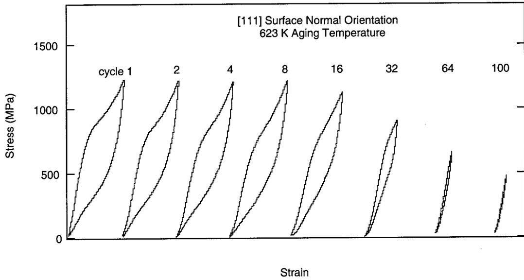
Figure 30: Compressive response of [111] oriented NiTi aged at 623 K
