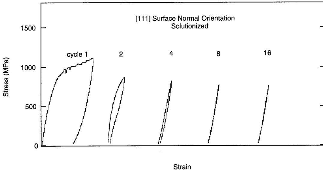
Figure 29: Compressive response of [111] oriented solutionized NiTi
