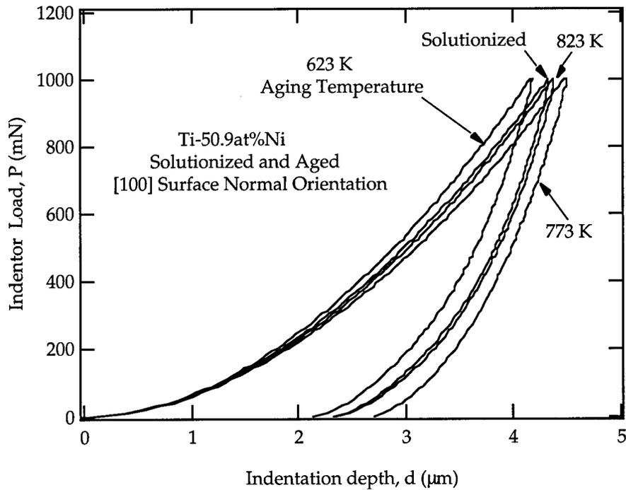
Figure 15: Loading curves for the [100] orientation.
