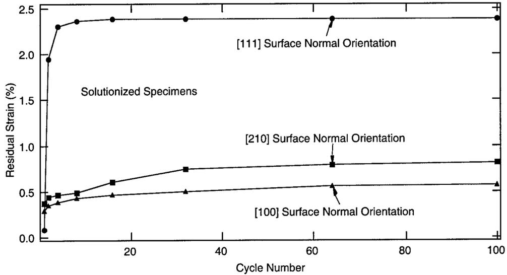
Figure 35: Residual strain accumulation for solutionized [100], [210], and [111] specimens
