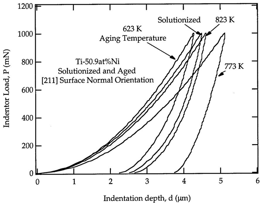
Figure 18: Loading curves for the [211] orientation.
