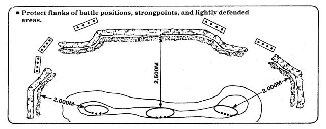
Tank ditches must complement natural terrain obstacles and other reinforcing (manmade) obstacles.
