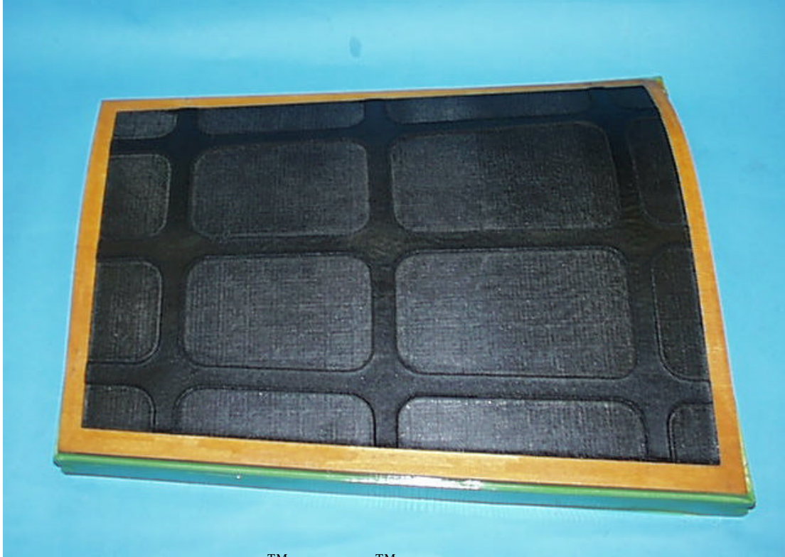
Figure 3.3.2-9 Pyrolyzed Nextel™/Blackglas™ Blastshield Demonstration Component 1.
