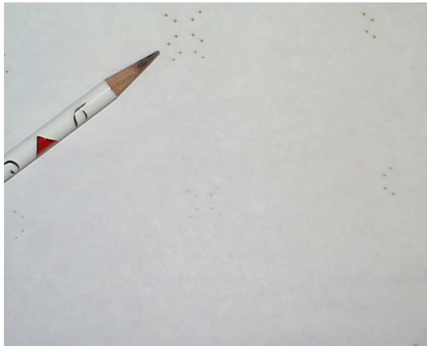
Figure 3.2.2-12 Example of laser calibration shots on LOM paper used for Inter-Regional Calibration procedure.
