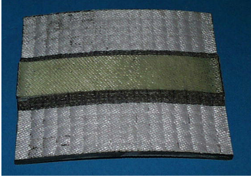
Figure 3.2.3-9 Green State 4"x 4" Curved Panel with edge/surface irregularities due to laser char zone
