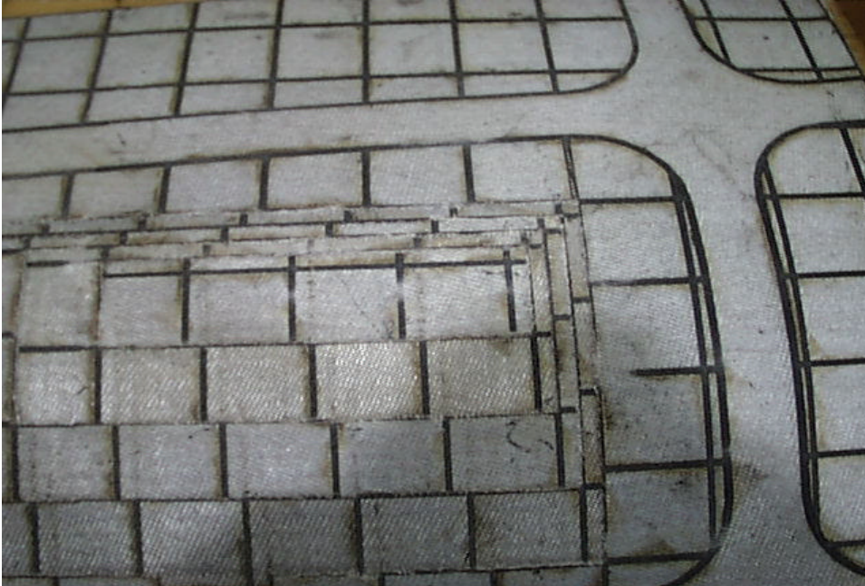
Figure 3.3.2-6 Partially decubed section of cured blastshield showing offset decube pattern
