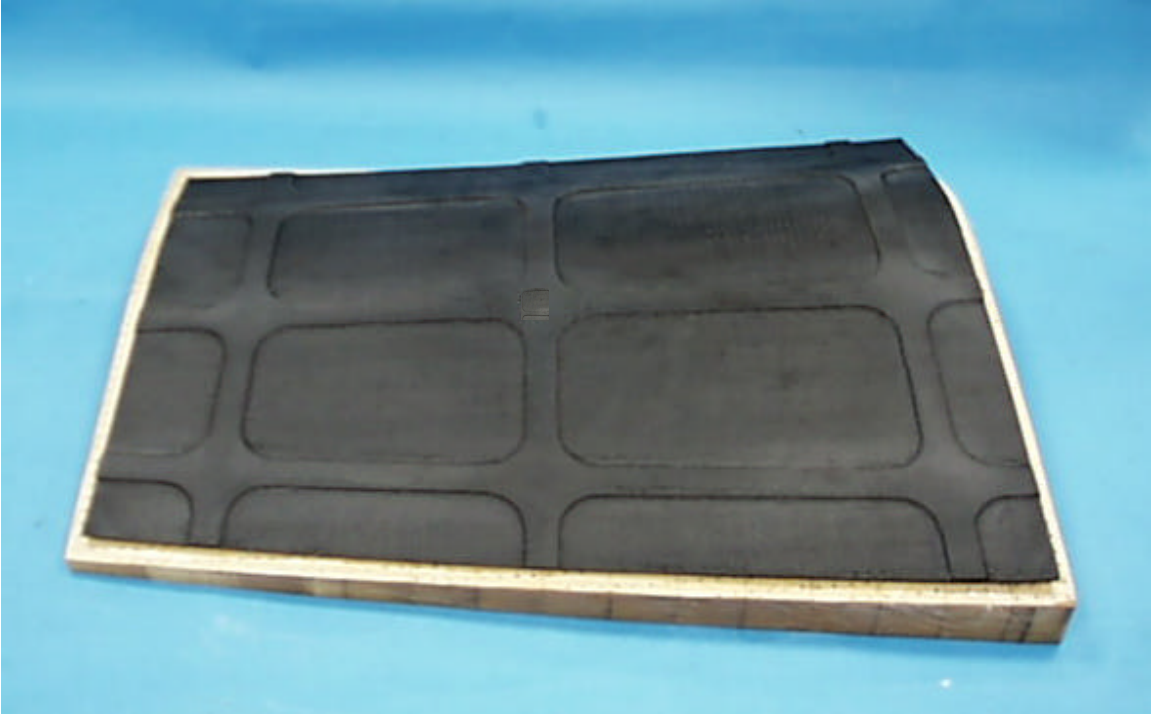
Figure 3.3.2-13 Nextel™/Blackglas™ Blastshield Demonstration Component 2 after pyrolysis.
