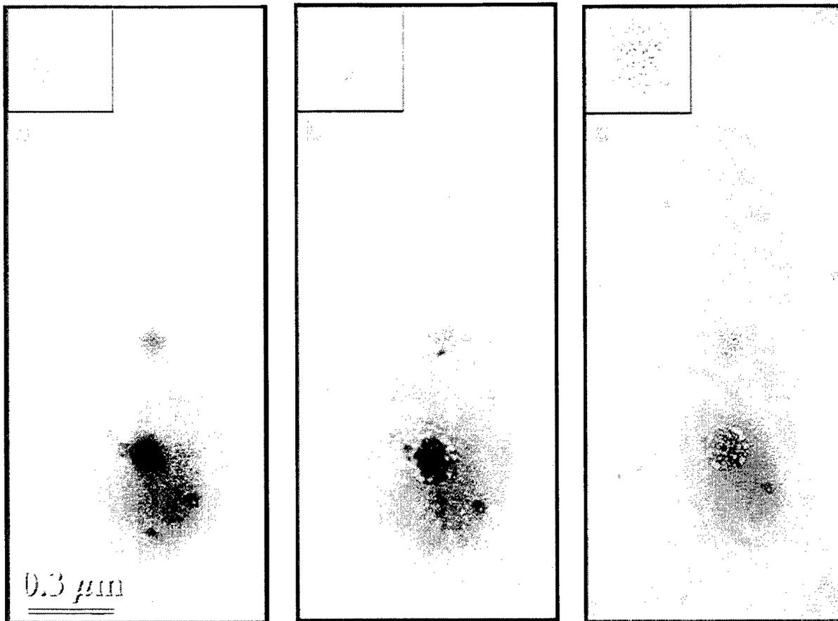
Figure 8. Series of images of hydrated *Pseudomonas putida* in the EC at 100 torr as a function of time (several minutes). Progressive electron beam damage to the nucleoid region is evident. Insert is a higher magnification of the nucleoid area.
