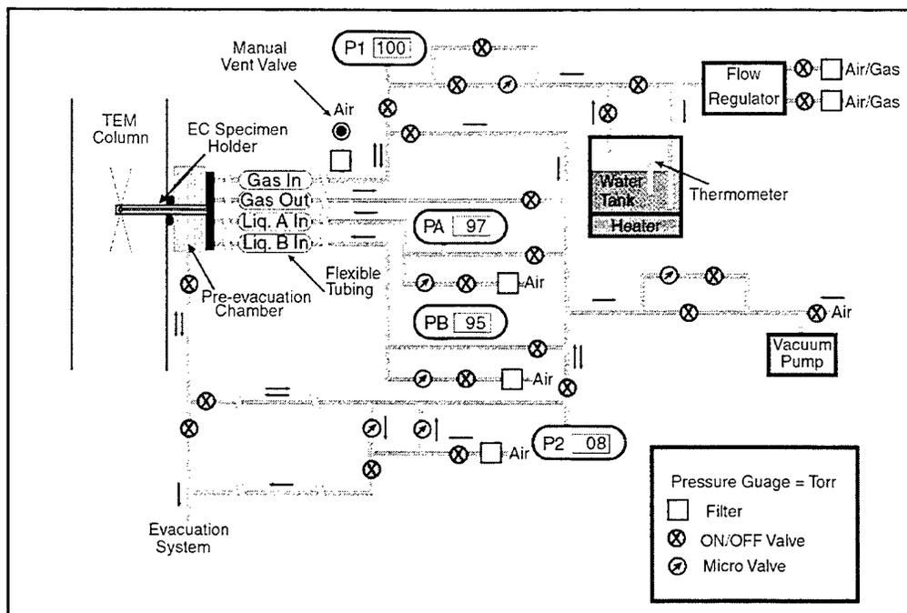
Figure 4. Diagrammatic representation of the EC control system.
