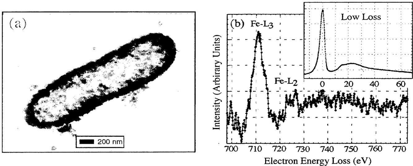
Figure 10. (a) *Pseudomonas putida* in the EC at 100 torr after removal of excess moisture by circulation of dry air through the environmental chamber. The cell is encrusted with electron dense particulates. (b) EELS spectrum from the bacteria demonstrate the presence of Fe based on the presence of the L<sub>3</sub> and L<sub>2</sub> core loss features of Fe. The core-loss regime spectrum is pre-edge background subtracted and deconvolution was used to remove plural scattering.
