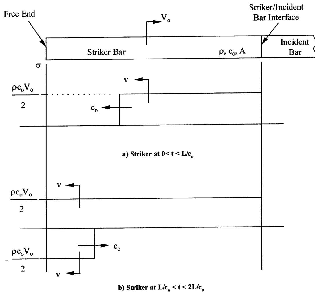
Figure 3.3 Stress waves propagating through striker bar
