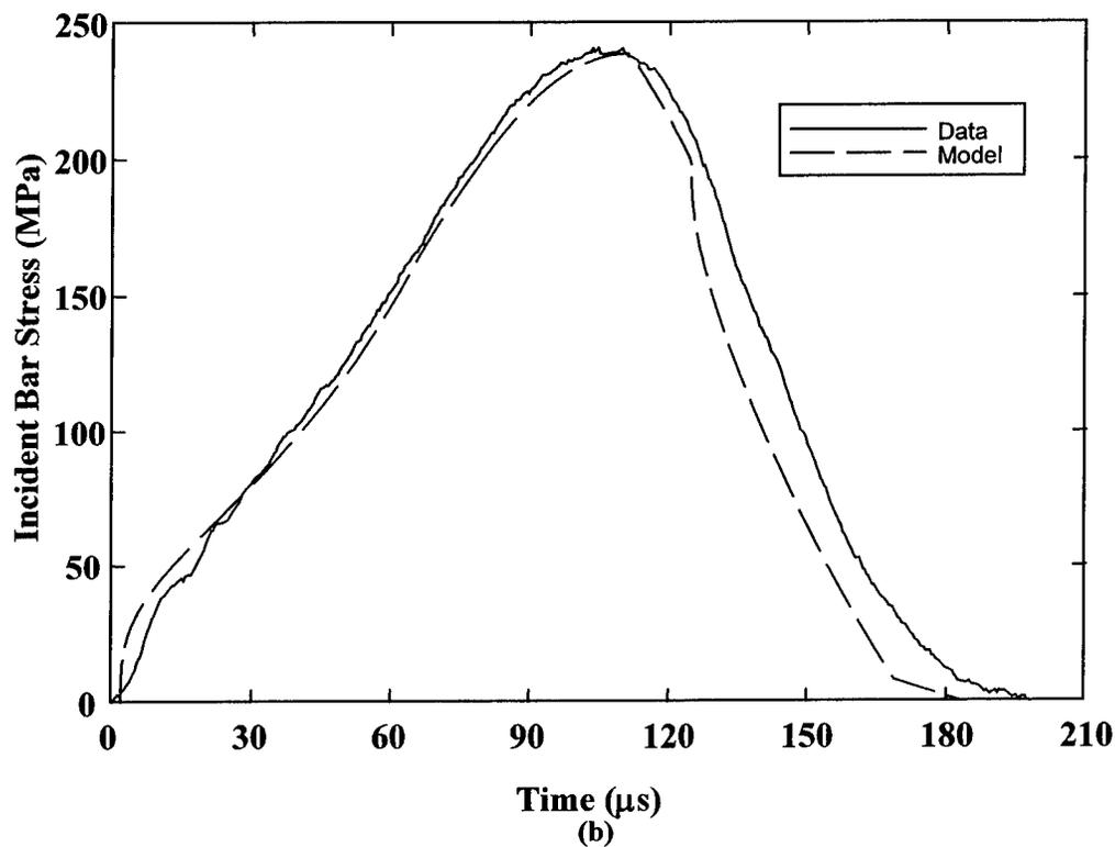
Figure B.12 Data and model predictions for nominal 4.8-mm-diameter by 1.6-mm-thick (a) hard and (b) annealed C11000 copper pulse shaper impacted by a 152.4-mm-long striker at a nominal velocity of 17.5 m/s
