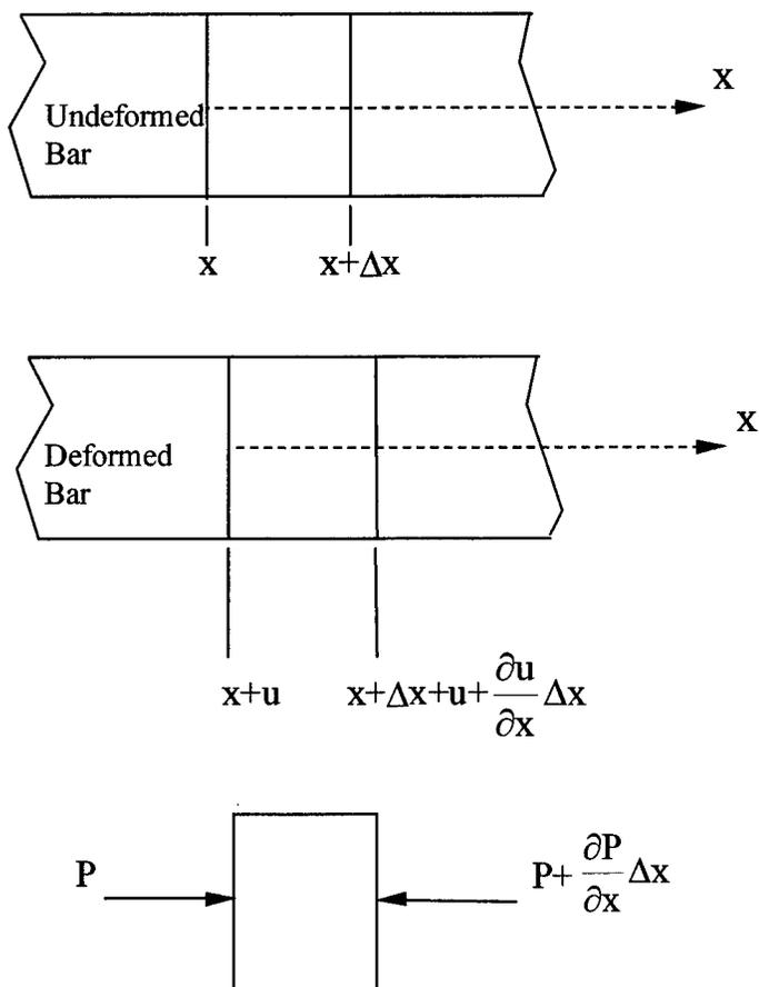
Figure 3.1 Differential element in cylindrical bar
