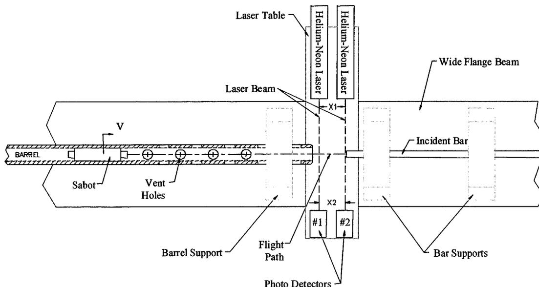
**Figure 3.8 Schematic of laser velocity measurement system**
