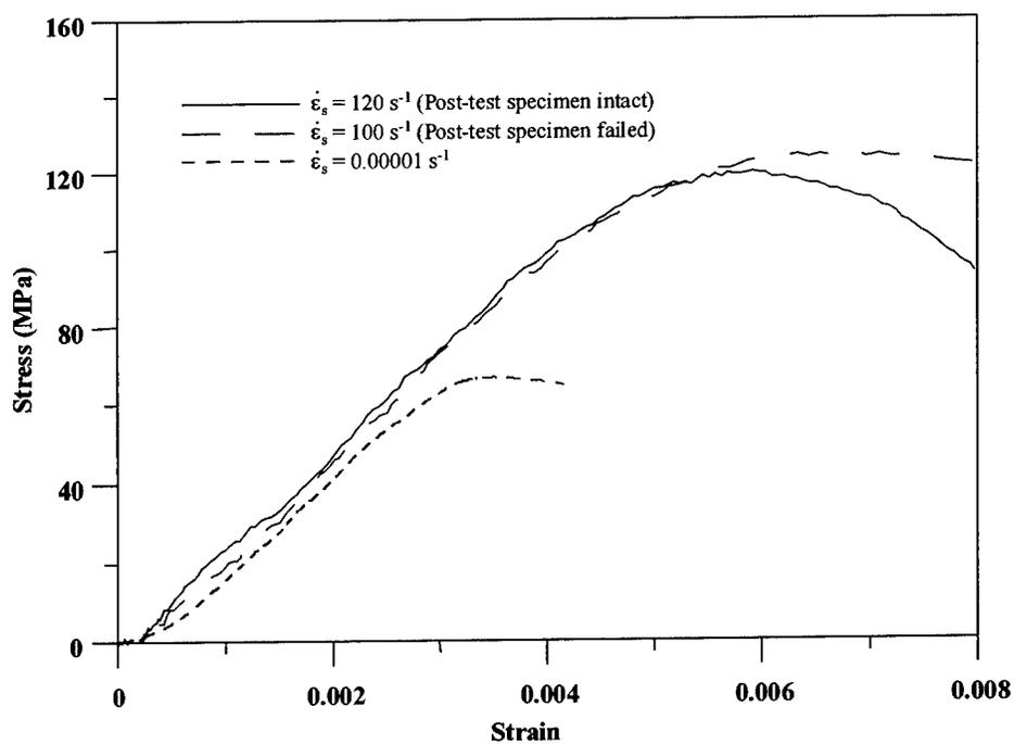
Figure 6.11 Quasi-static and dynamic stress-strain limestone data
