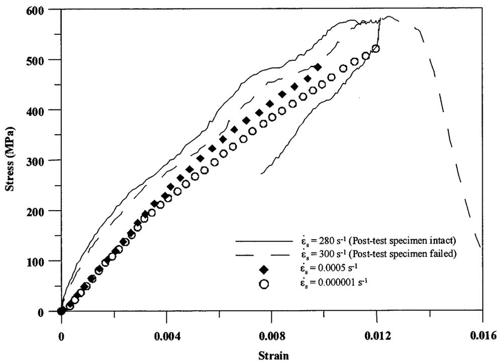
Figure 7.7 Quasi-static and dynamic stress-strain data for Macor
