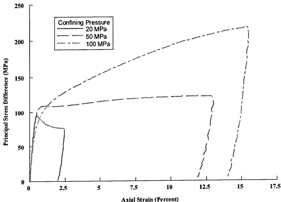
**Figure 2.1 Batch 3 limestone triaxial compression data**
