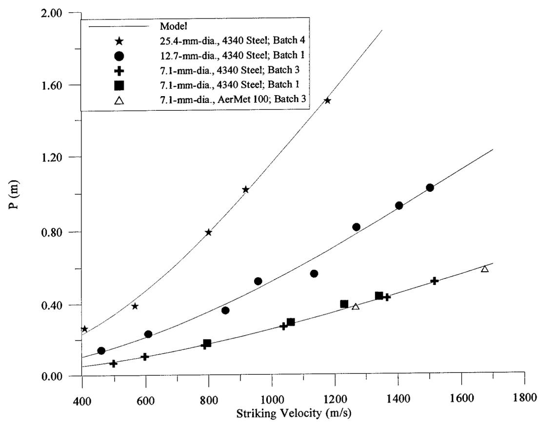
Figure 2.4 Data and model predictions for limestone targets
