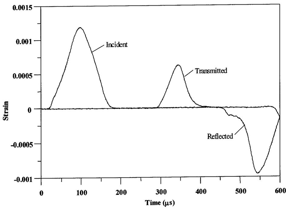
Figure 6.7 Strain-time signals for a pulse shaped SHPB experiment with a limestone sample
