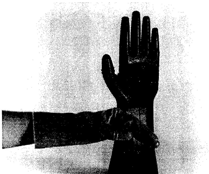
Figure 4. Rapid prototyping form of an early glove design used to dip prototype gloves for design verification.
