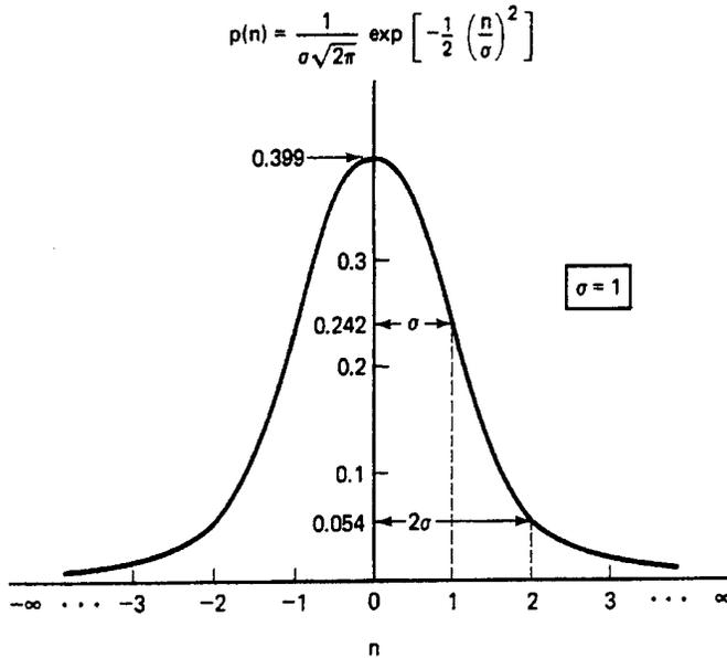
Figure 14. Normalized ( $\sigma=1$ ) Gaussian Probability Density Function.
