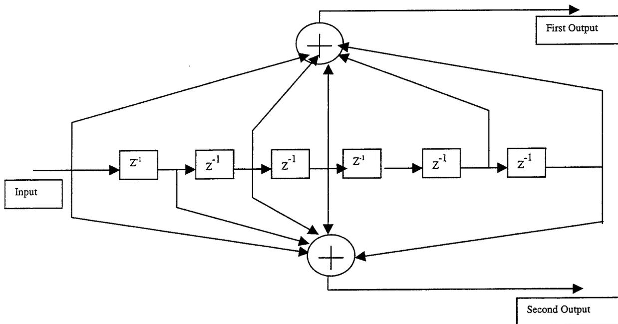
Figure 2. Convolutional Encoder.
