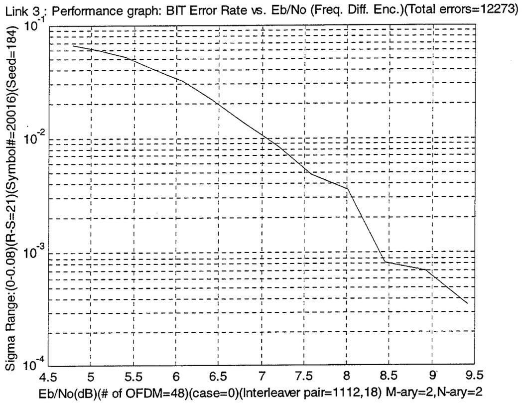
Figure 50. COFDM DBPSK Modulation With Model 3 Link 3.
