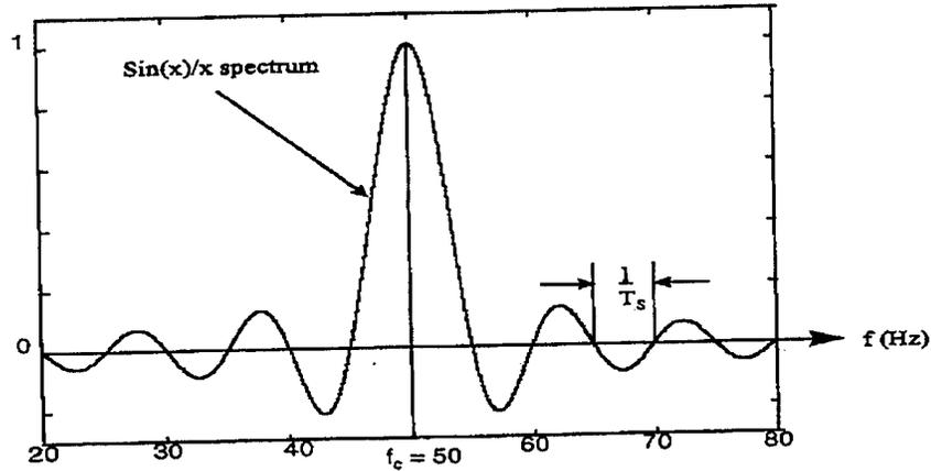
Figure 7. Spectrum For Single Symbol With Length  $T_s$ .
