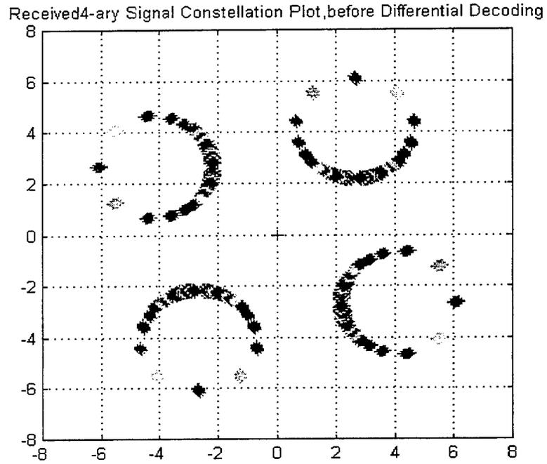
Figure 39. Signal Constellation Plot Before Differential Decoding.
