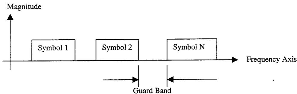
Figure 5. Additional Guard Band In Frequency Spectrum.
