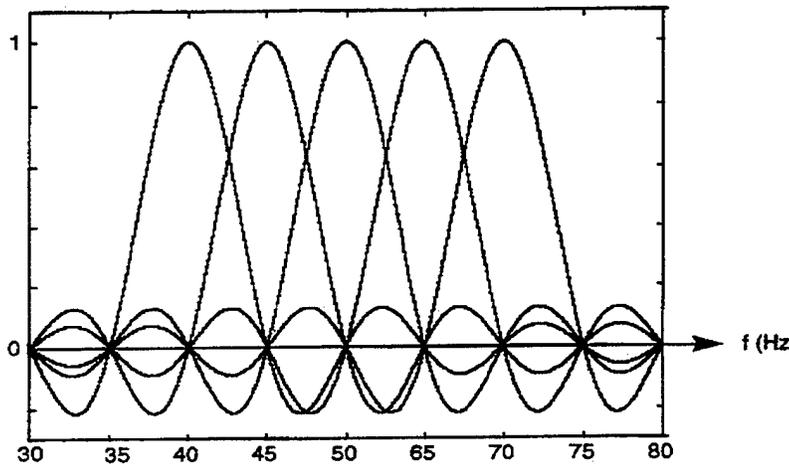
Figure 8. OFDM Spectrum.
