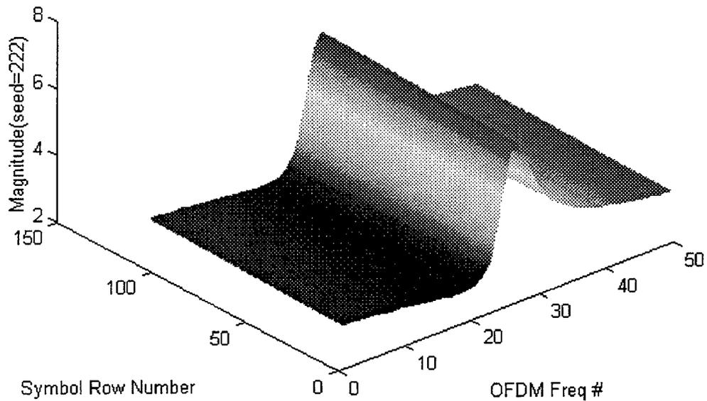
Figure 41. Received Signal With Frequency Selective Fading.
