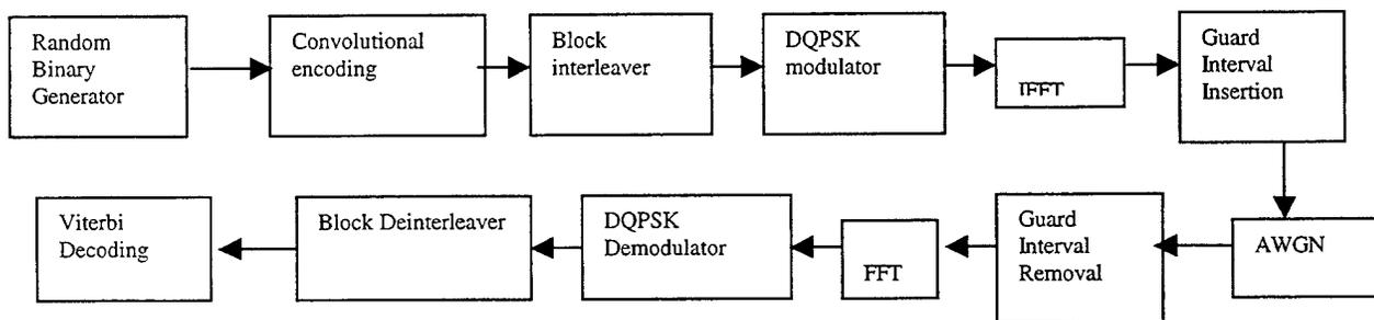
Figure 1. Basic Configuration Of a Coded OFDM Model.
