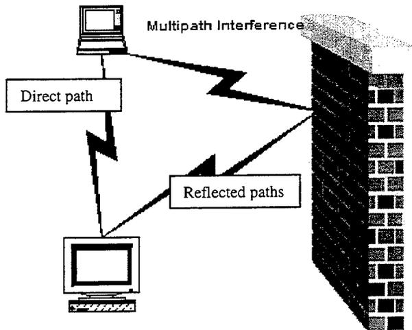
Figure 16. Multipath Interference.
