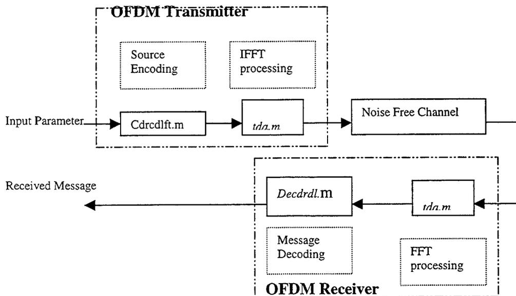
Figure 25. Emulation Of The COFDM Communication System.
