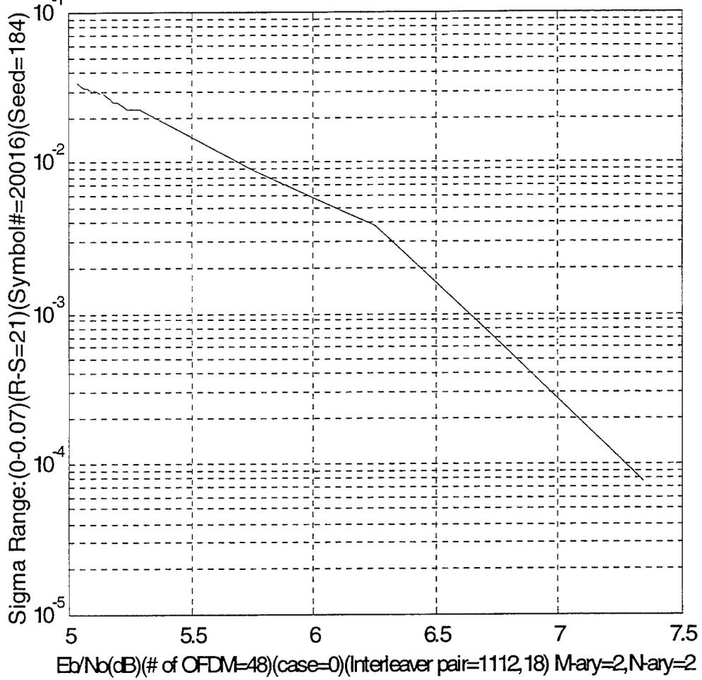
Figure 47. COFDM DBPSK Modulation With Model 1 (AWGN).
