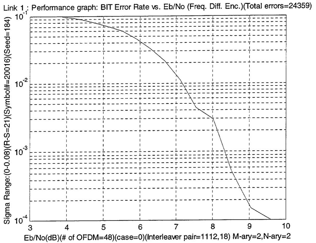
Figure 48. COFDM DBPSK Modulation With Model 3 Link 1.
