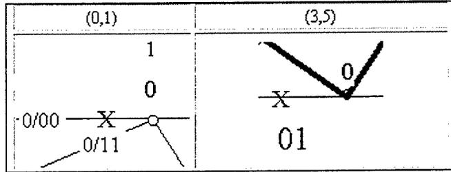
Figure 13. Extract Of Viterbi Trellis Diagram In Figure 12.
