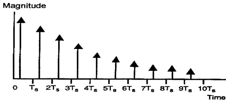
Figure 19. Channel Impulse Response For IEEE 802.11a.
