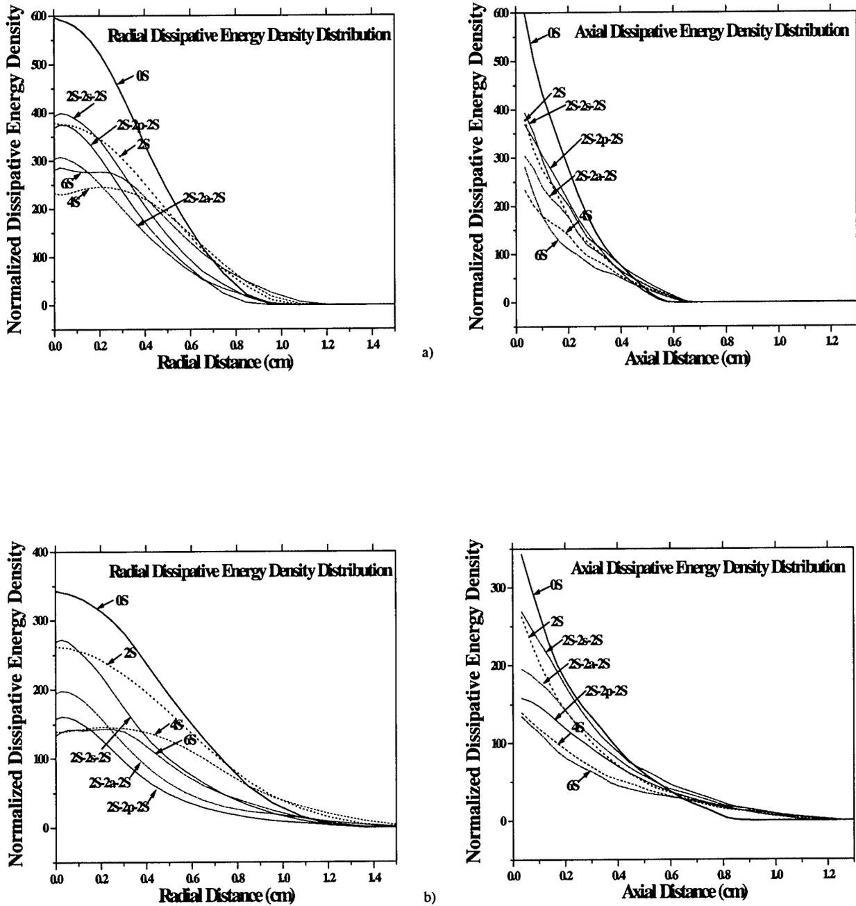
Figure 3: Radial and axial distribution of normalized dissipative energy density in an aluminum substrate for various SiC layering configurations. The damage of SiC is suppressed. The shock front is at, (a) 1 cm, and (b) 2 cm, into the substrate.
