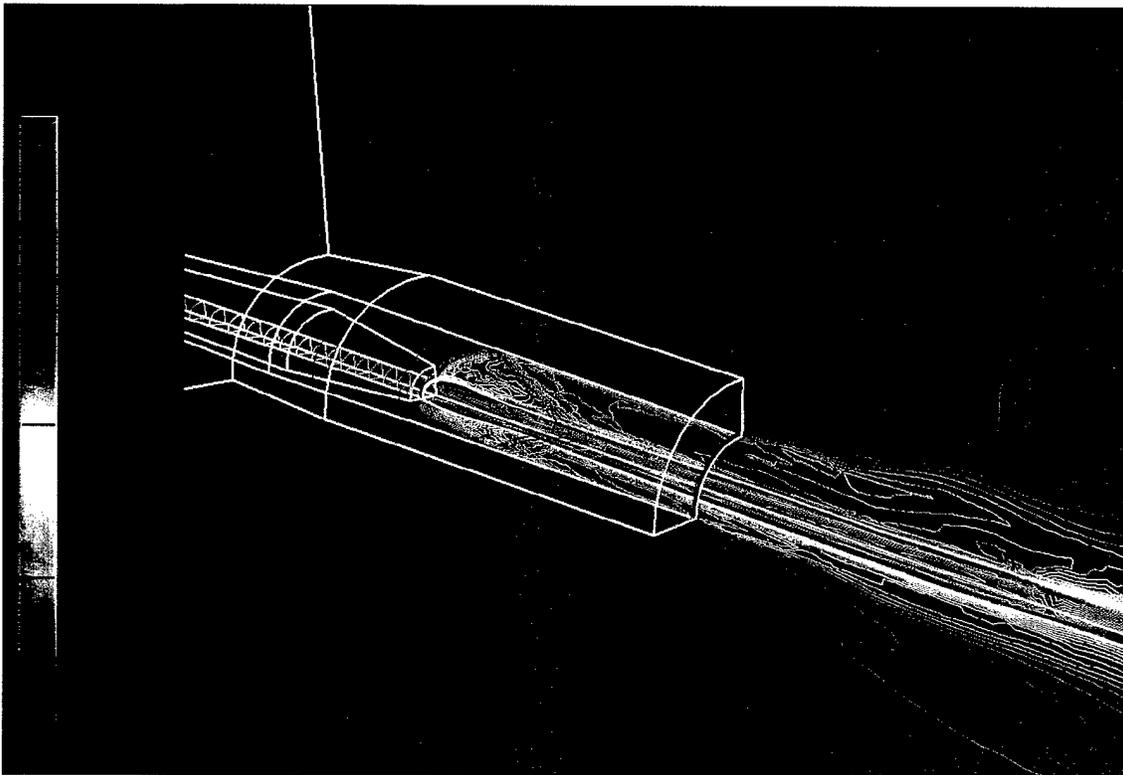
Figure 17. Flow through nozzle with capillary moved in 10.0mm,
