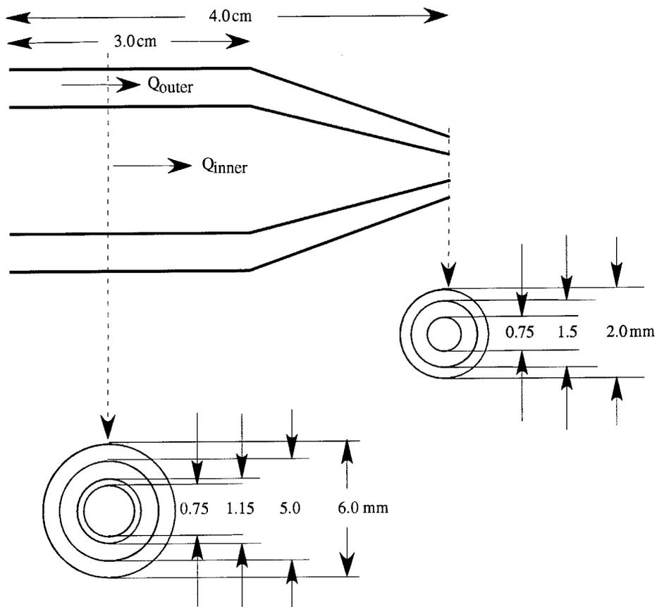
Figure 1. Nozzle geometry
