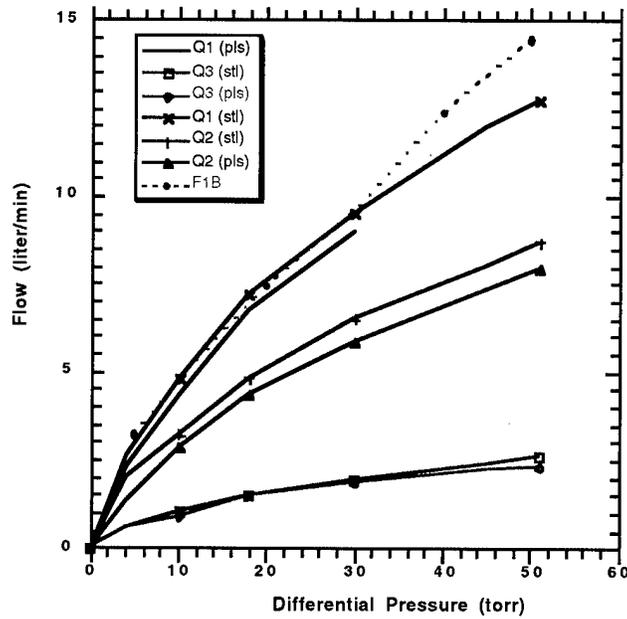
Figure 5. Experimental pressure drop across the nozzle
