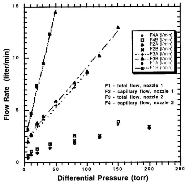
Figure 2. Experimental pressure drop for a similar nozzle
