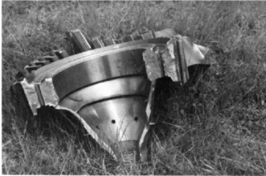
Fig. 1: Largest fragment of fan hub after burst (Pensacola accident)
