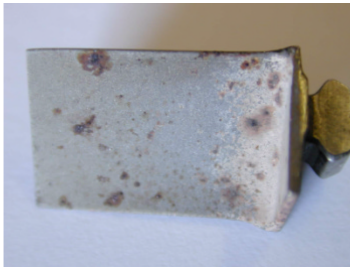
Fig. 6 – Pitting Corrosion on a HH-3F Compressor Blade
