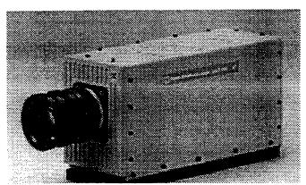
camera is capable of recording up 2000 frames per second. With a total recording time of 2.73 seconds (5,461 images) this camera allows us to capture the delayed structure response under blast/impact loading. Another valuable aspect of this camera is that it has a continuous loop type of recording setup. Because of this type of recording, images can be captured both in the pre and post trigger stages.
