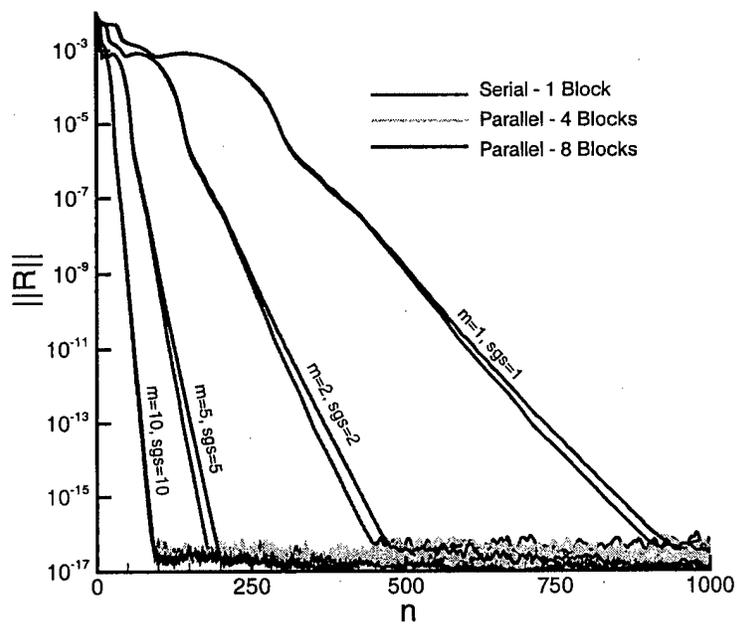
Figure 9: Convergence history using the SGS method to invert the implicit operator on a parallel computer. The results from a serial computer are plotted for comparison.  $n$  is the number of physical time iterations,  $m$  is the number of pseudo time subiterations, and  $sgs$  is the number of iterations of the SGS method.
