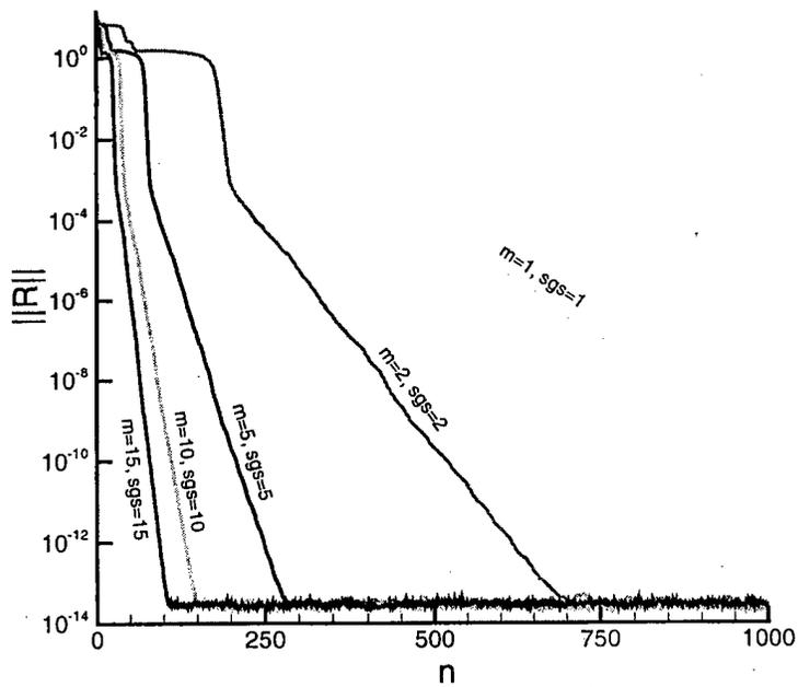
Figure 6: Convergence history using the SGS method to invert the implicit operator.  $n$  is the number of physical time iterations,  $m$  is the number of pseudo time subiterations, and  $sgs$  is the number of iterations of the SGS method.
