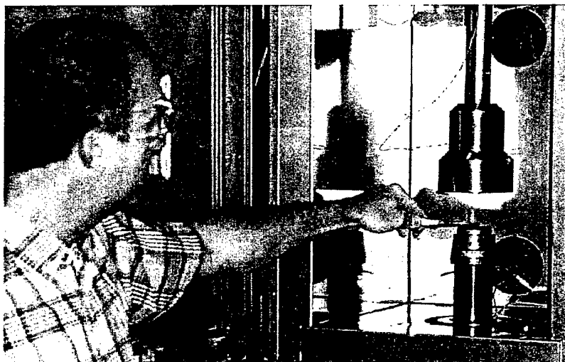
Figure 3. Energetic material prepared for testing on the MTS load frame.
