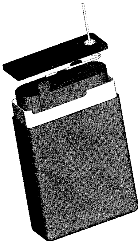
Fig. 2. A cross-section view of the coiled electrode configuration (A). An assembly view of a typical battery with the cover and electrode coil partially removed showing the attachments in the headspace (B).
