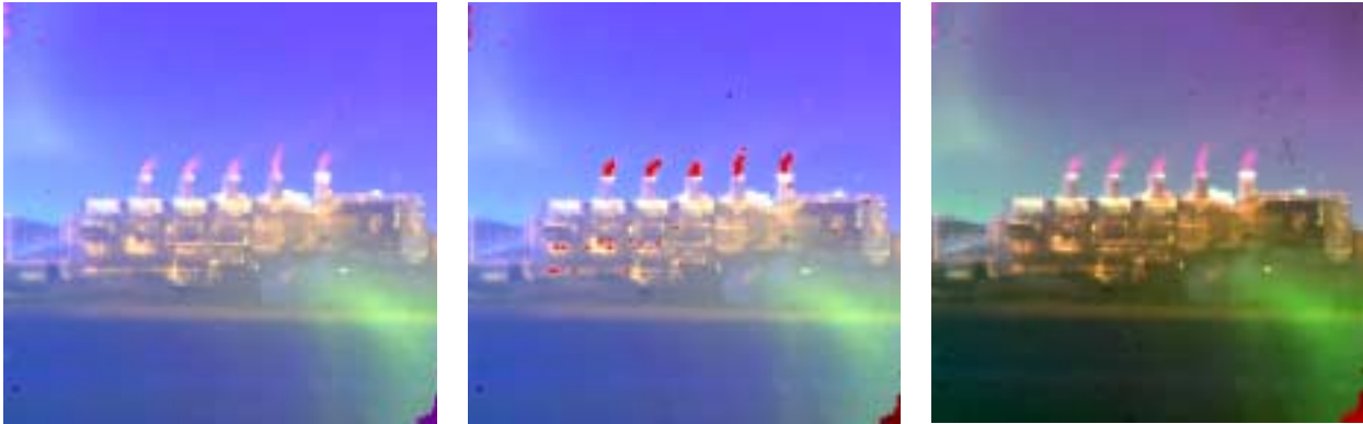
Figure 3. The system can compare three fusion algorithms simultaneously in real-time. The left image is created using Simple Color Fusion, the middle image with Red Enhancement, and the right image with Principle Component Fusion. There is glint on the lens apparent in the shorter of the two midwave bands, the green band. In the Red Enhancement, image pixels in the face of the power plant that were slightly red are presented with maximum red value. In the Principle Component image, the difference between the color of the sky, power plant, glint, and water in front of the plant is accentuated.
