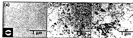
Fig. 2. PTEM image of a-Si films annealed at 650 °C for 3 hours. The C_O in each a-Si is (a) 5 \times 10^{21} , (b) 8 \times 10^{20} , and (c) 5 \times 10^{20} /cm 3 , respectively.
