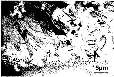
Figure 1: Plane view TEM micrograph of an Ar + - laser crystallized polycrystalline Si. Single scanned trace on a glass substrate. The grains, that grow fastest and laterally overgrow others are 2-10 μm in width. The grain boundaries are oblique, 40° to the scan direction. Nanocrystals at the rim from explosive crystallization are visible.
