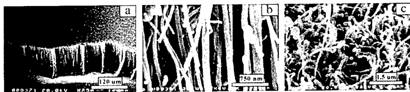
Figure 1. SEM micrograph of well aligned carbon nanotubes grown with gas flow rate of 40 sccm at 950 °C for 10 min on a large area (20 mm ×30 mm) of Co-Ni codeposited Si substrates. (a) A uniformly distributed morphology of vertically aligned carbon nanotubes, (b) magnified side view of (a), (c) top view of the vertically aligned carbon nanotubes.
