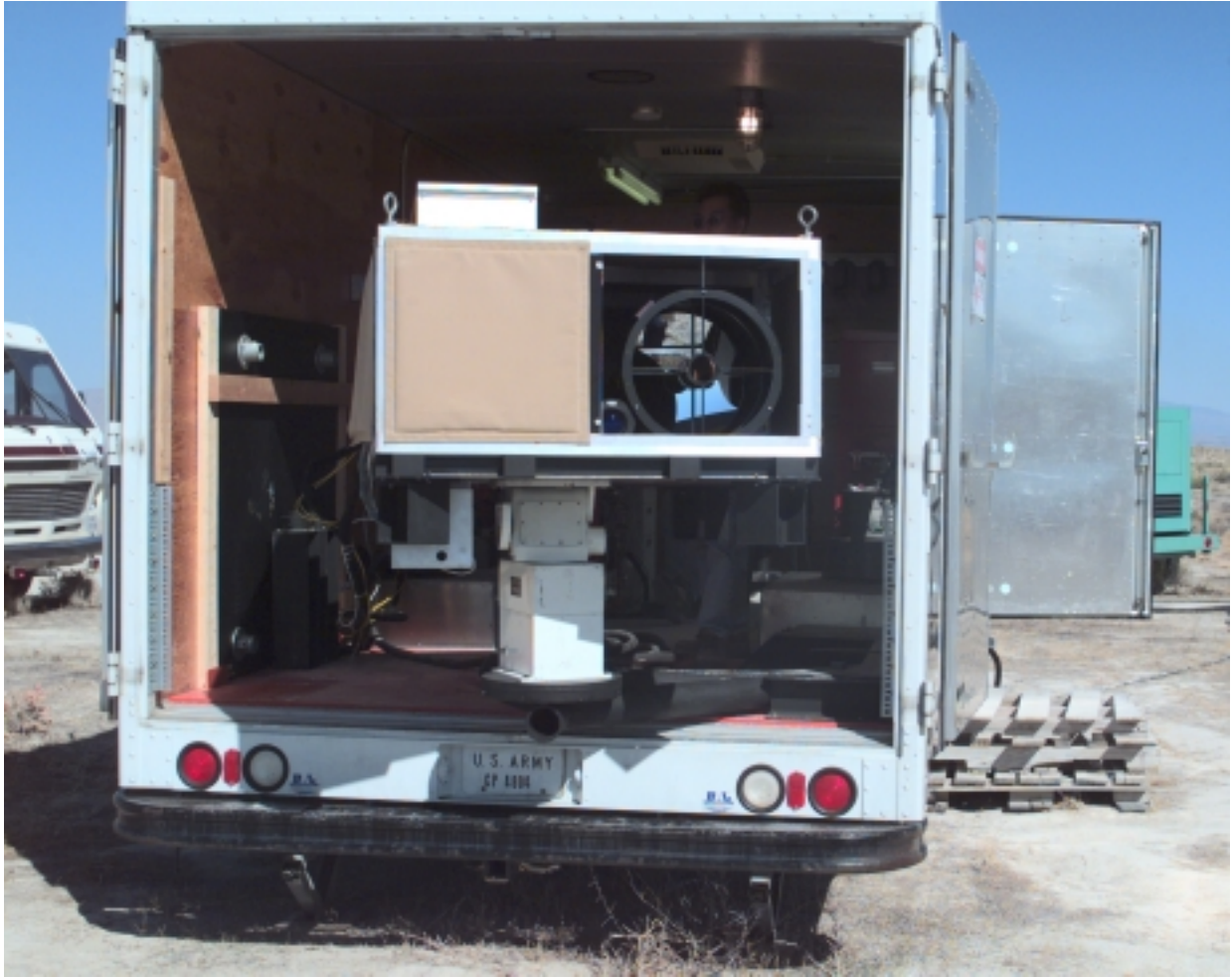
Figure 2: FAL Lidar, manufactured by Raytheon (formerly Hughes Aircraft Company).
