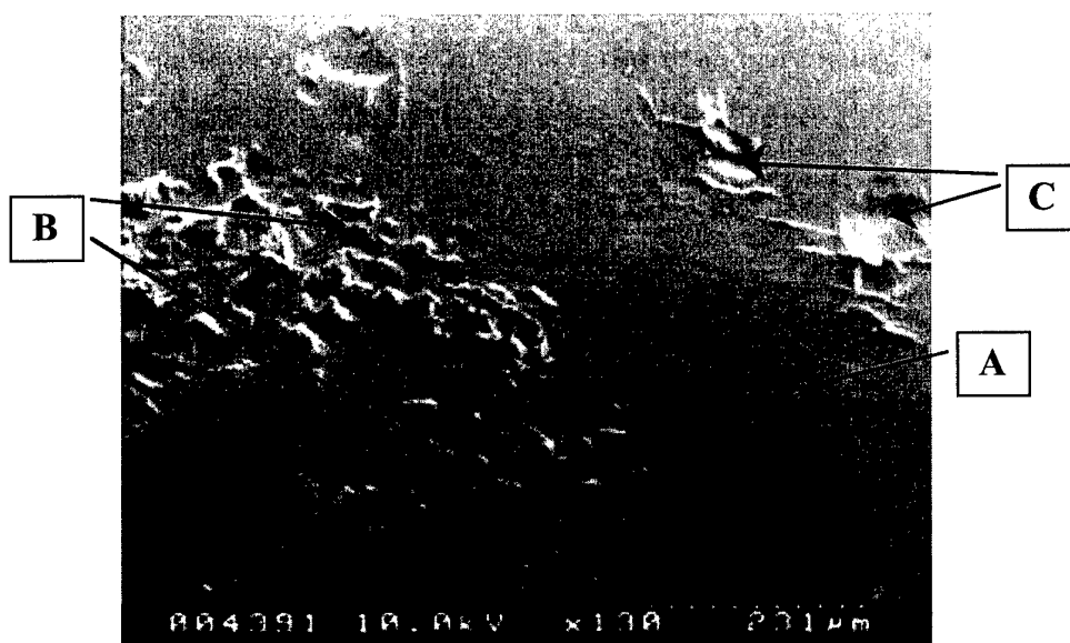
Fig. 10 SEM image of a Y-oriented LGS LPE film surface.
