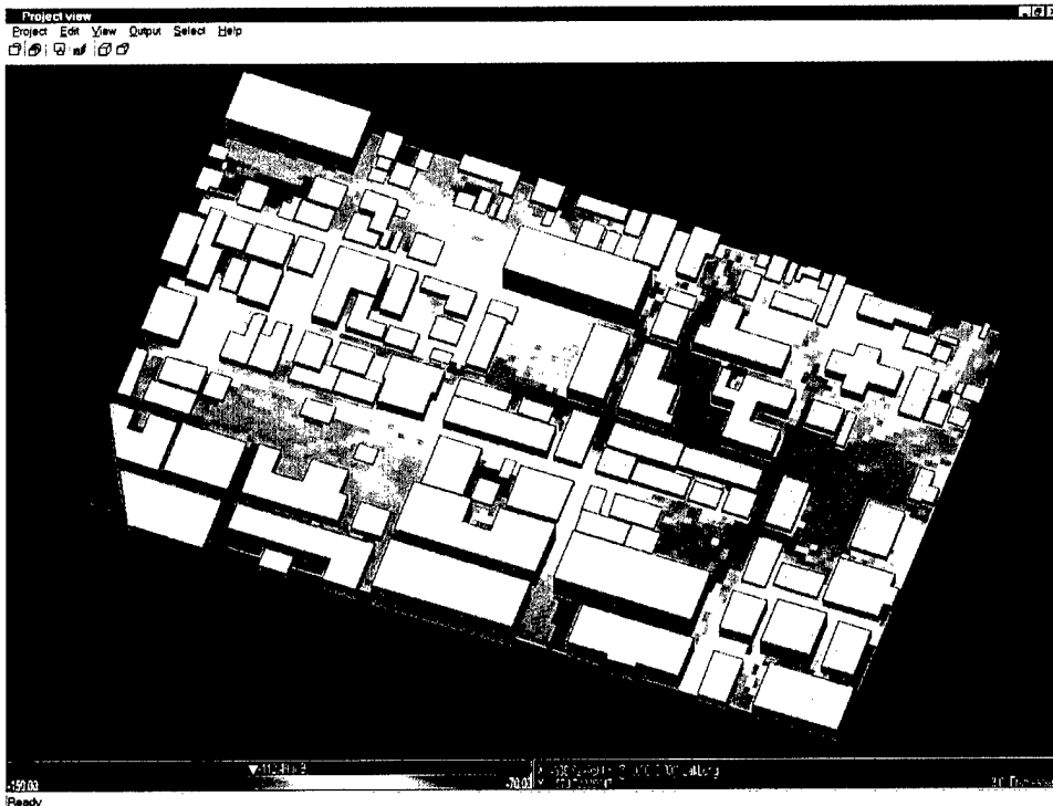
Figure 16 Coverage area display illustrating the Point-to-Multipoint capability of Wireless InSite.
