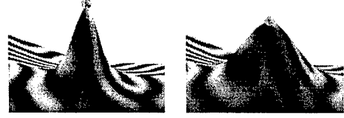
Figure 4: Illustration of Changing Mask Scale: Exaggerated pulling deformations clearly illustrate different spatial scales in the underlying traction distribution. In each case, pressure masks were automatically generated using the linear spherical mask functional (see §3.1.3) for different values of the radius parameter, r . This example shows (left) a single vertex mask, and (right) a mask involving several nearby vertices. Note that in each case the surface has been once refined using Loop subdivision.
