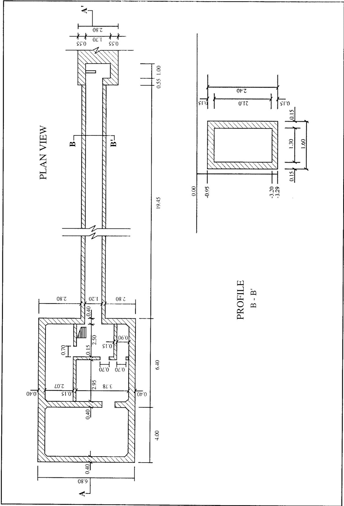
Figure 20. Plan drawing of the "Force Protection" guard house, and associated tunnel and entry structures. Derzhavinsk, Regiment 2, Silo 3. All measurements are in meters.
