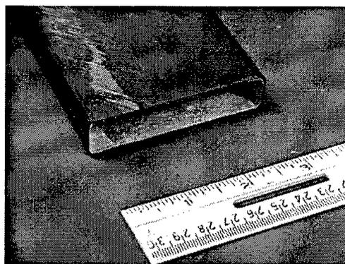
Figure 13 Composite box beam
