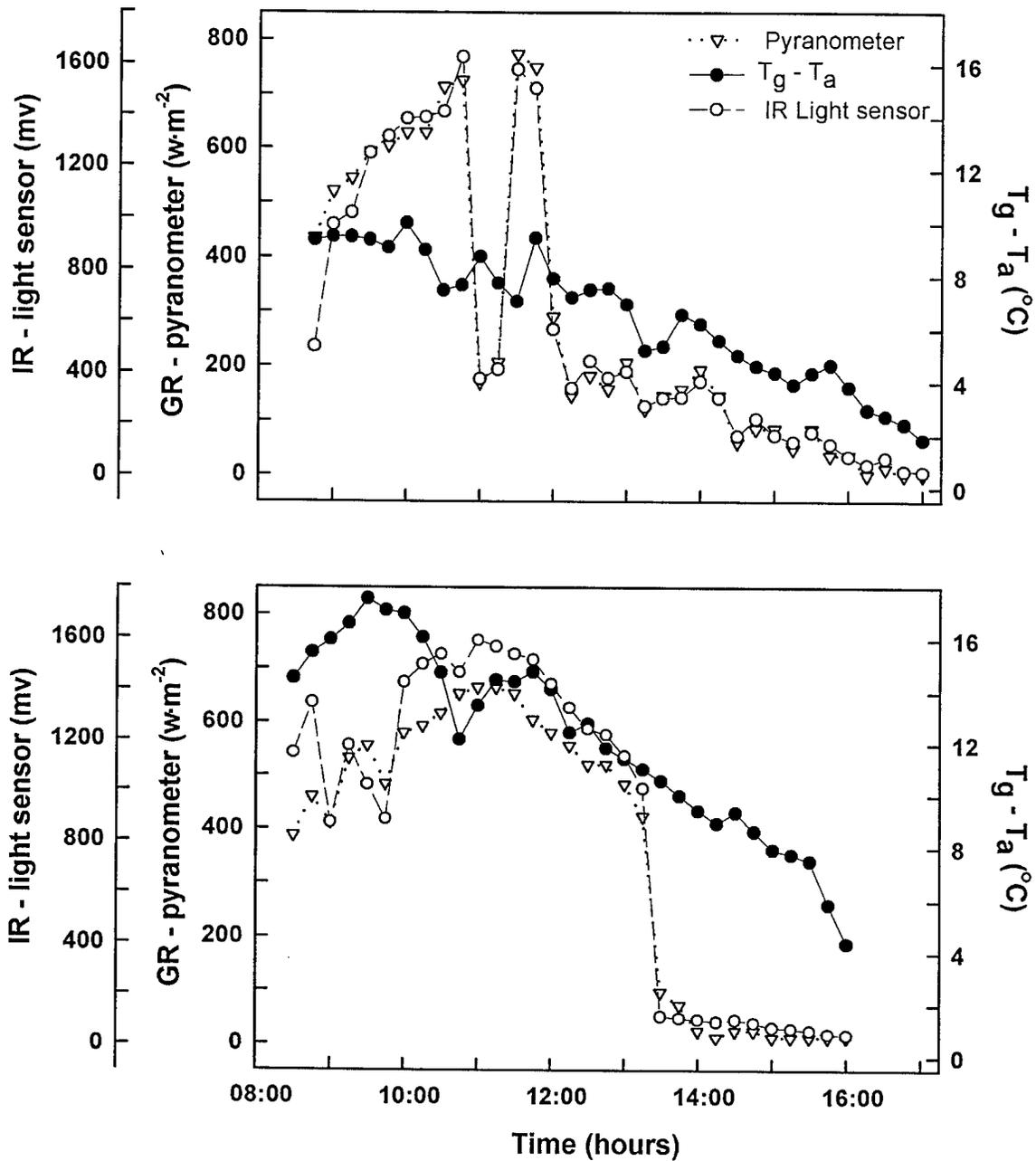
Figure 6. Global radiation (GR) measured by pyranometer, black globe thermometer ( $T_g$ ) and infra-red (IR) sensor during two partly cloudy days. Data showing the  $T_g$  did not reflect the GR in the morning (top) and lagged behind the change to overcast in the afternoon (bottom).
