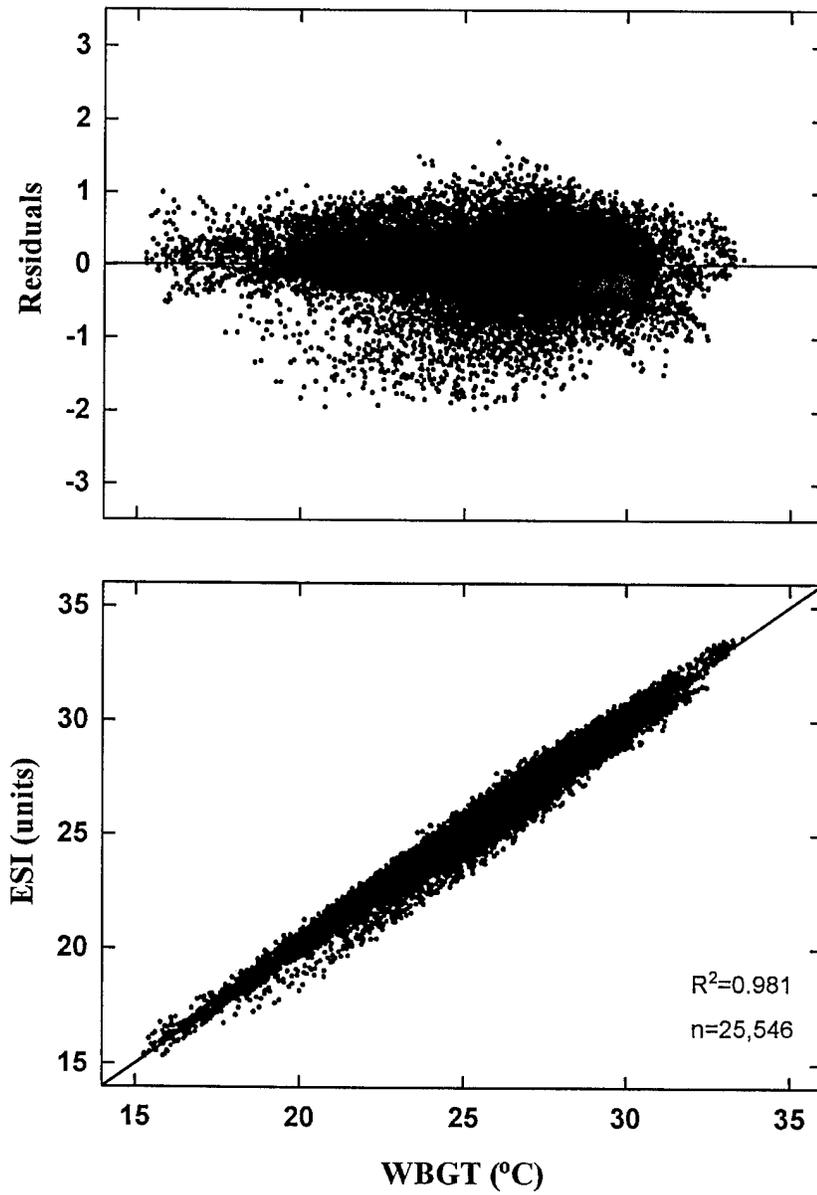
Figure 5. Comparison of suggested ESI with the WBGT index showing correlation (bottom) and residuals scattergram (top). Database for this figure was collected from 16 different locations.
