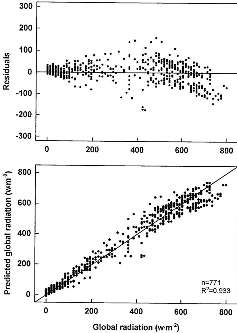
Figure 8. Comparison of the PGR with global radiation measured by pyranometer. Data showing residuals scattergram by the time of the day.
