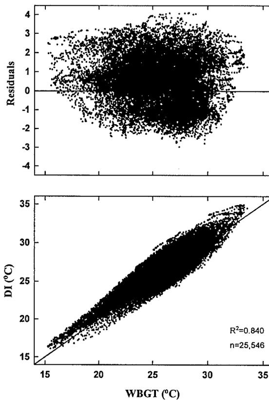
**Figure 1. Comparison of DI [18] with the WBGT index showing correlation (bottom) and residuals scattergram (top).**
