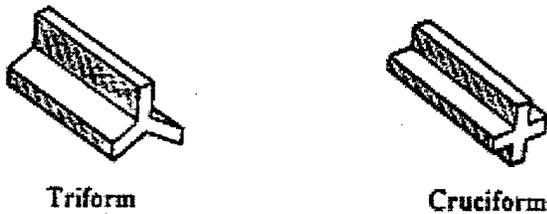
**Figure 5. Novel Penetrator Geometries From Bless et al. (1995).**
