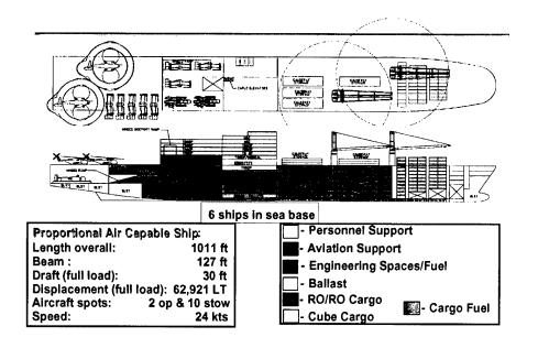
Figure 57. AME Ship Design for MPF-F Option C
