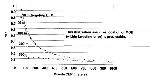
Figure 13. Probability of a Ballistic Missile Hitting the MOB
