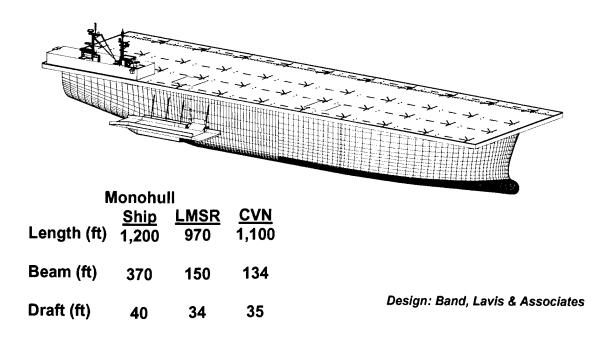
Figure 19. Notional Monohull Ship Alternative to MOB for Sea Base
