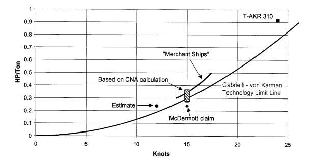
Figure 27. HP/Ton vs Maximum Speed
