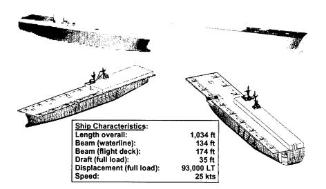
Figure 58. BLA Ships Designed for MPF-F
