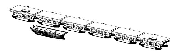
Figure 20. Relative Size of Monohull Sea Base and a 6-SBU MOB
