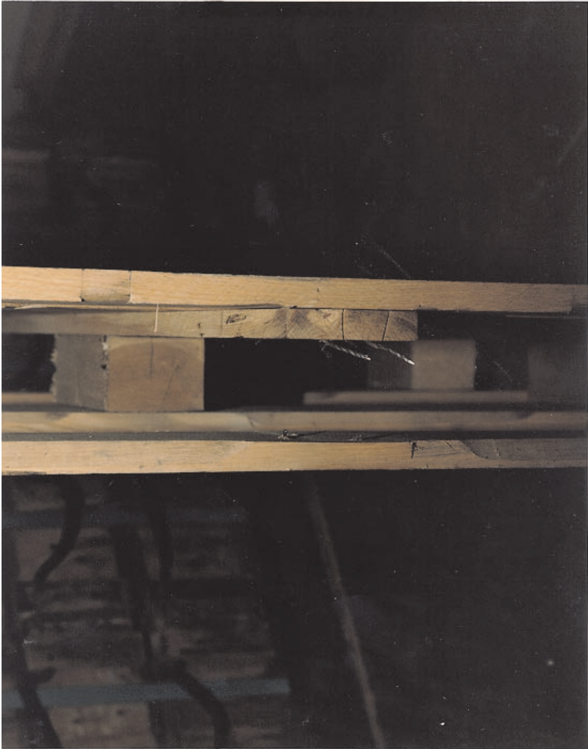
U.S. ARMY DEFENSE AMMUNITION CENTER AND SCHOOL - SAVANNA, IL AO317-SCN96-37-838. This photo shows the location where one of the posts of Stewart's Forest Products, Inc. pallet no. 5 pulled away from during the edgewise rotational drop test.
