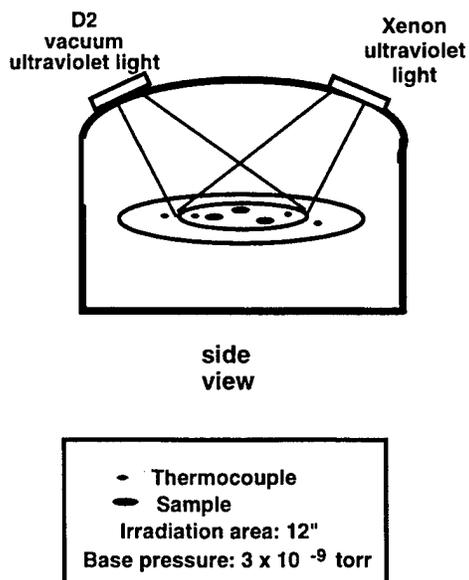
Figure 1. The Space Environmental Effects Chamber.
