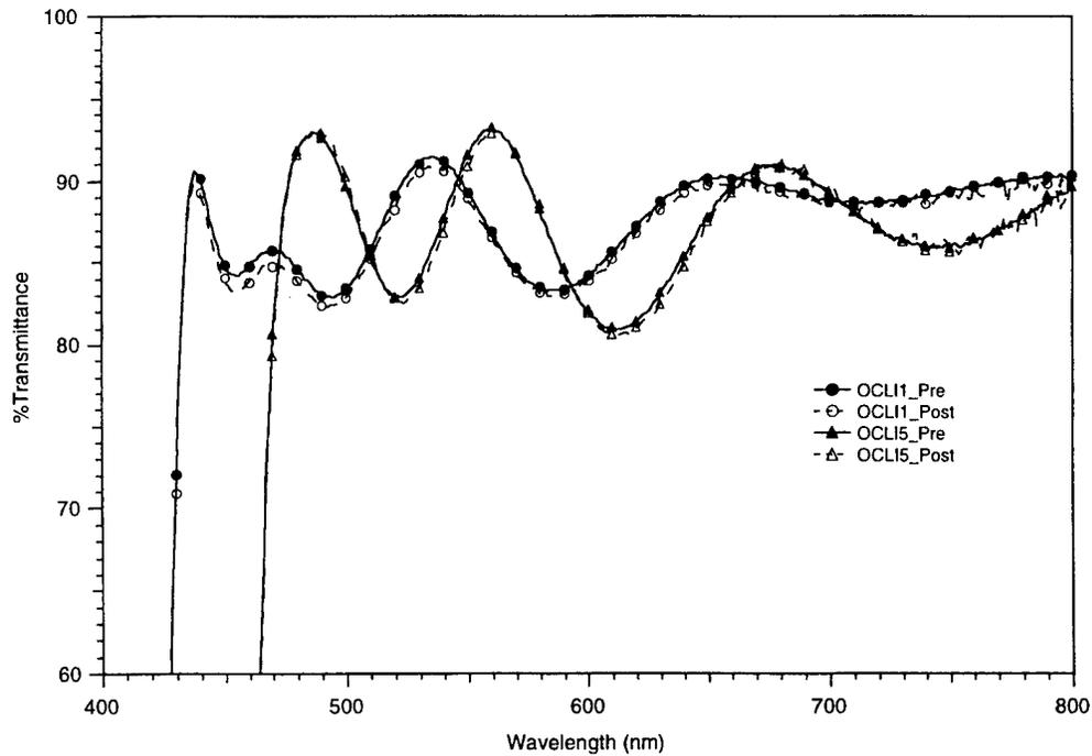
Figure 7. Plot of sample transmission before and after UV exposure for two OCLI-coated fused-silica samples: (1) New  $ZrO_2/SiO_2$  configuration, (5) Old  $Ta_2O_5/TiO_2/SiO_2$  configuration.
