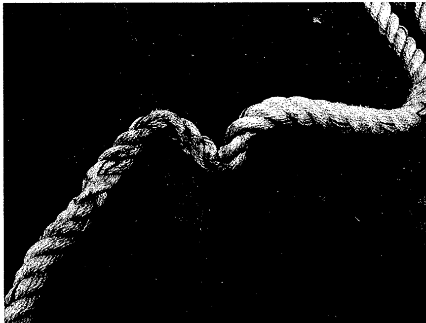
Figure 12: At the location of the former bow-line knot permanent deformation of the rope is found. Two permanent pressure points are seen in the center and the lower left of the image.
