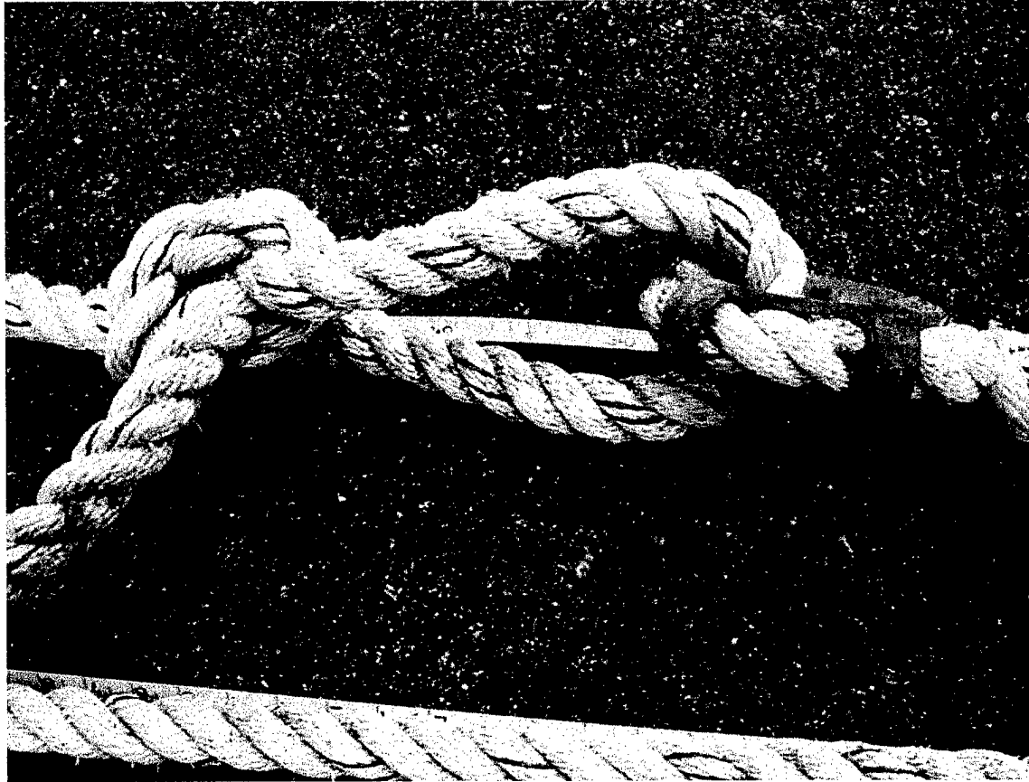
Figure 10: Bowline knot tie-in to thimbled rope eye in center of long-line after 19 months deployment at the WHOI Buoy Farm site.
