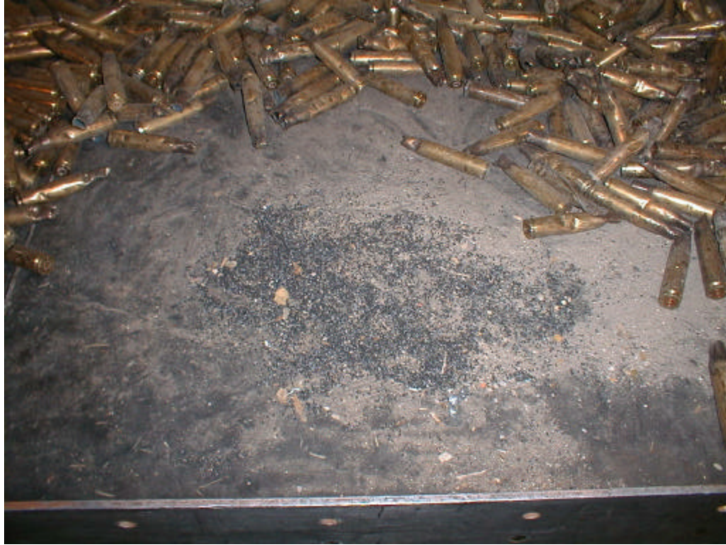
Photo 5. 1% Live Mixture of .50 Caliber Ammunition With Loose Propellant Processed Through CP Manufacturing, Inc., OD5000 Ordnance Deformer
