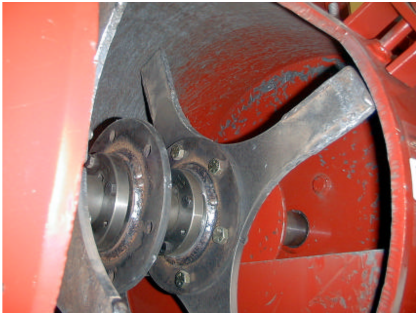
Photo 3. CP Manufacturing, Inc., OD5000 Ordnance Deformer, Showing the Deformer Drum Interior
