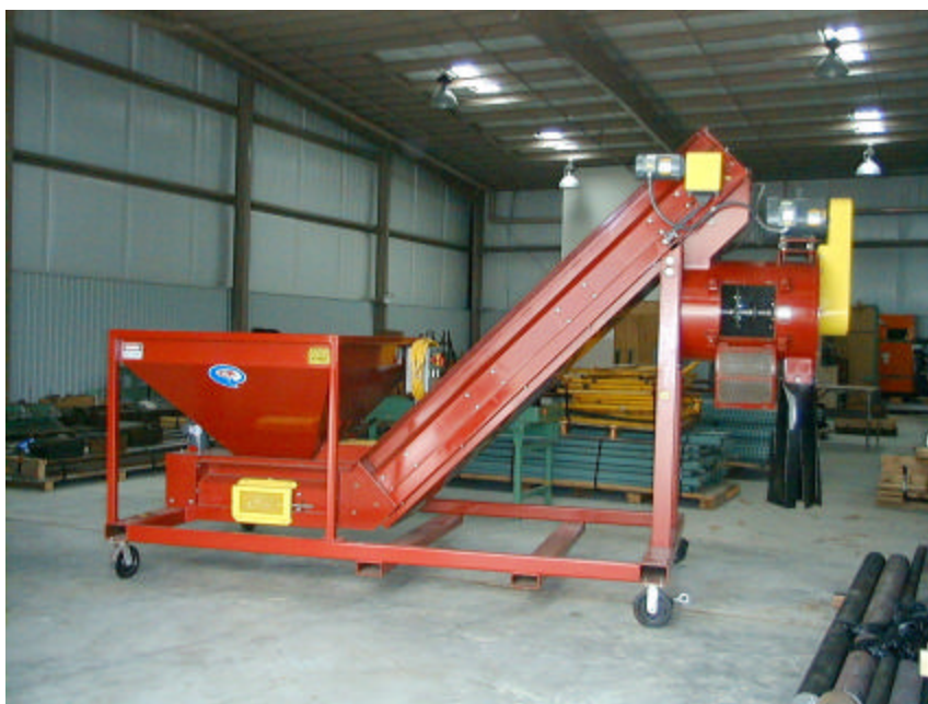
Photo 1. CP Manufacturing, Inc., OD5000 Ordnance Deformer, Showing Holding Bin, Conveyor, and Deformer Drum
