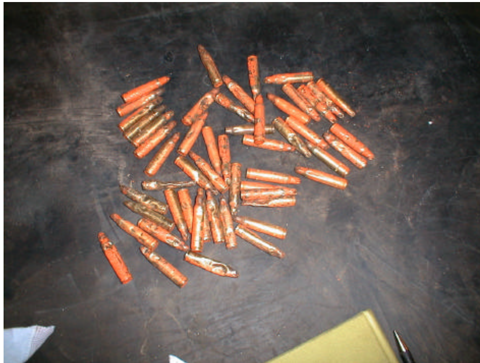
Photo 4. 1% Live Test With 5.56mm Blank Ammunition Processed Through the CP Manufacturing, Inc., OD5000 Ordnance Deformer
