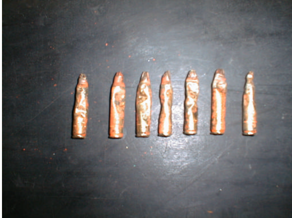
Photo 9. 1% Live Test with 5.56mm Blank Ammunition in Bouldin & Lawson Rotary Drum Ordnance Deformer
