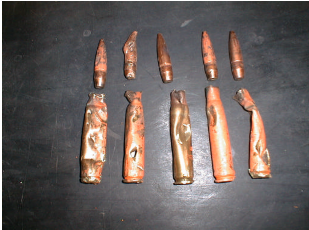
Photo 10. 1% Live Test With .50 Caliber Ammunition Processed Through Bouldin & Lawson Rotary Drum Ordnance Deformer
