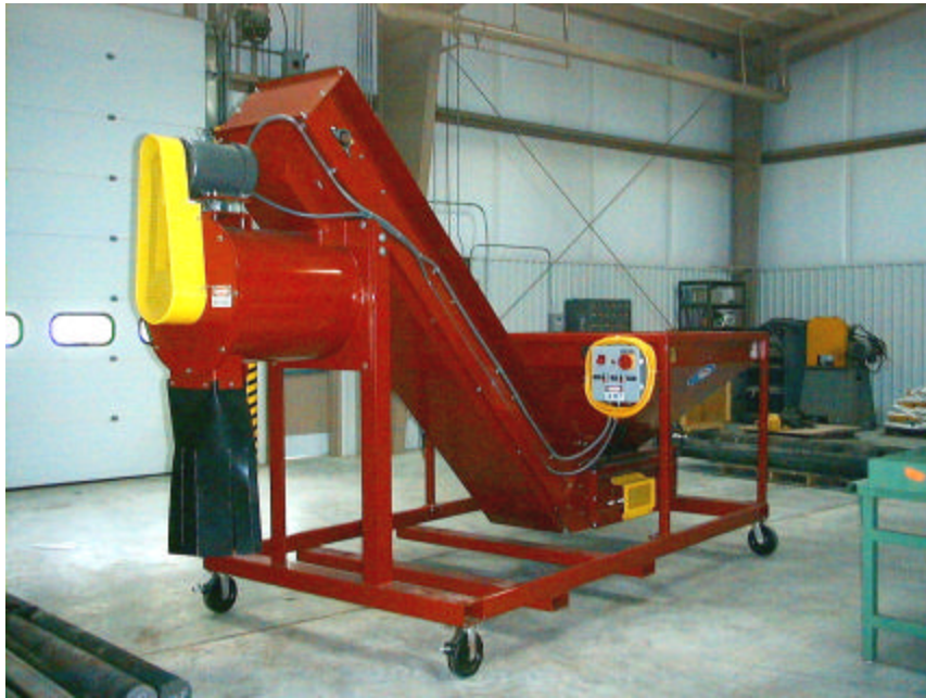
Photo 2. CP Manufacturing, Inc., OD5000 Ordnance Deformer, Showing the Deformer Drum and the Exit Chute
