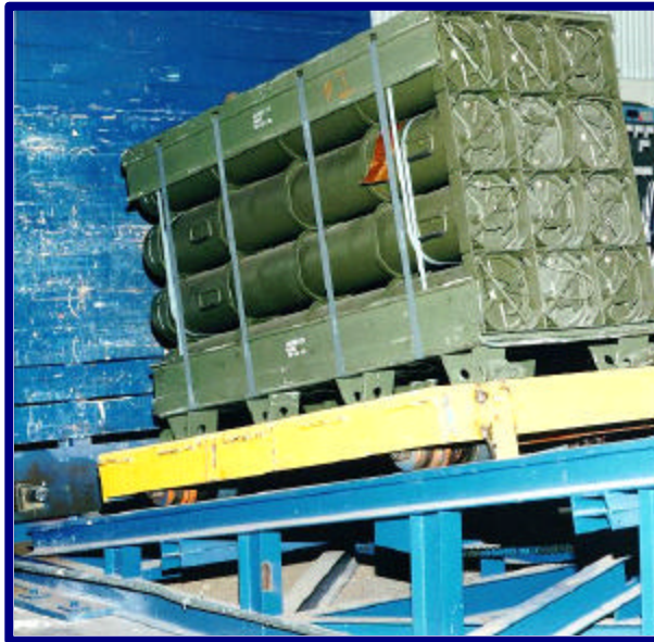
Figure 4. Example of the Incline-Impact Test. (2.75 Inch, Hydra 70, PA151 Rocket Pallet on incline-impact tester.)
