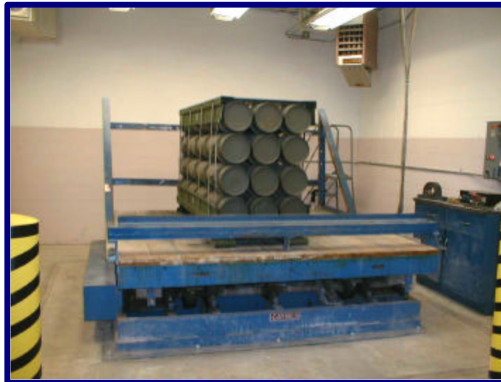
Figure 6. PA150 Hydra Test Pallet on the Vibration Table.
