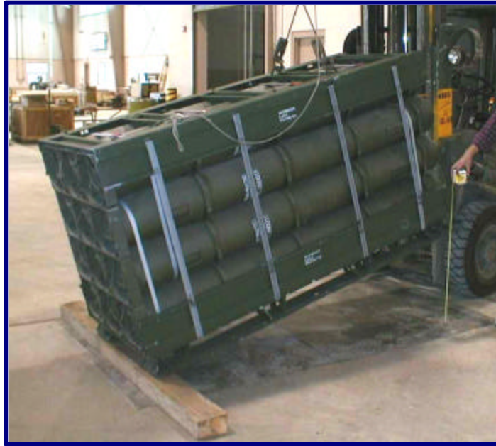
Figure 8. Edgewise Rotational Drop of Pallet No. 2
