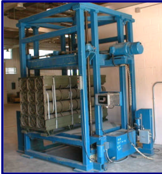
Figure 5. PA150 Hydra Test Pallet in the Compression Tester.
