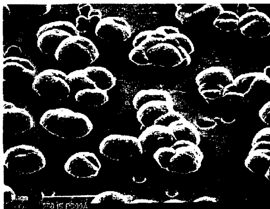
Fig. 17. Remaining structure after dissolution of the 10 \mu\text{m} porous polymeric filter. The Cu "mushrooms" were electrochemically deposited by cyclic potentiodynamic deposition from a copper pyrophosphate bath. The cyclic voltage was scanned at a rate of 500 mV/s.
