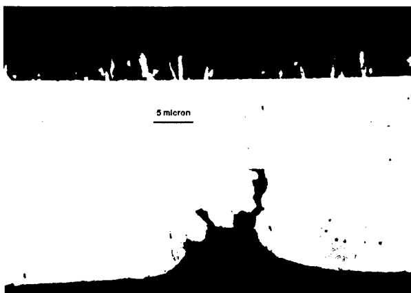
Fig. 13. Cross section showing the deposit as formed at a current density of 1 \text{ mA/cm}^2 for 7 hours followed by a current density of 5 \text{ mA/cm}^2 for between 1-2 hours. The cell configuration is that shown in Fig. 2A. The electrolyte is Cu pyrophosphate with the leveler. Electrodeposition was performed at room temperature.
