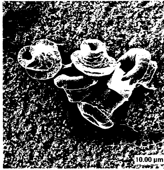
Fig. 12. Micrograph showing deposit after dissolving the membrane.
