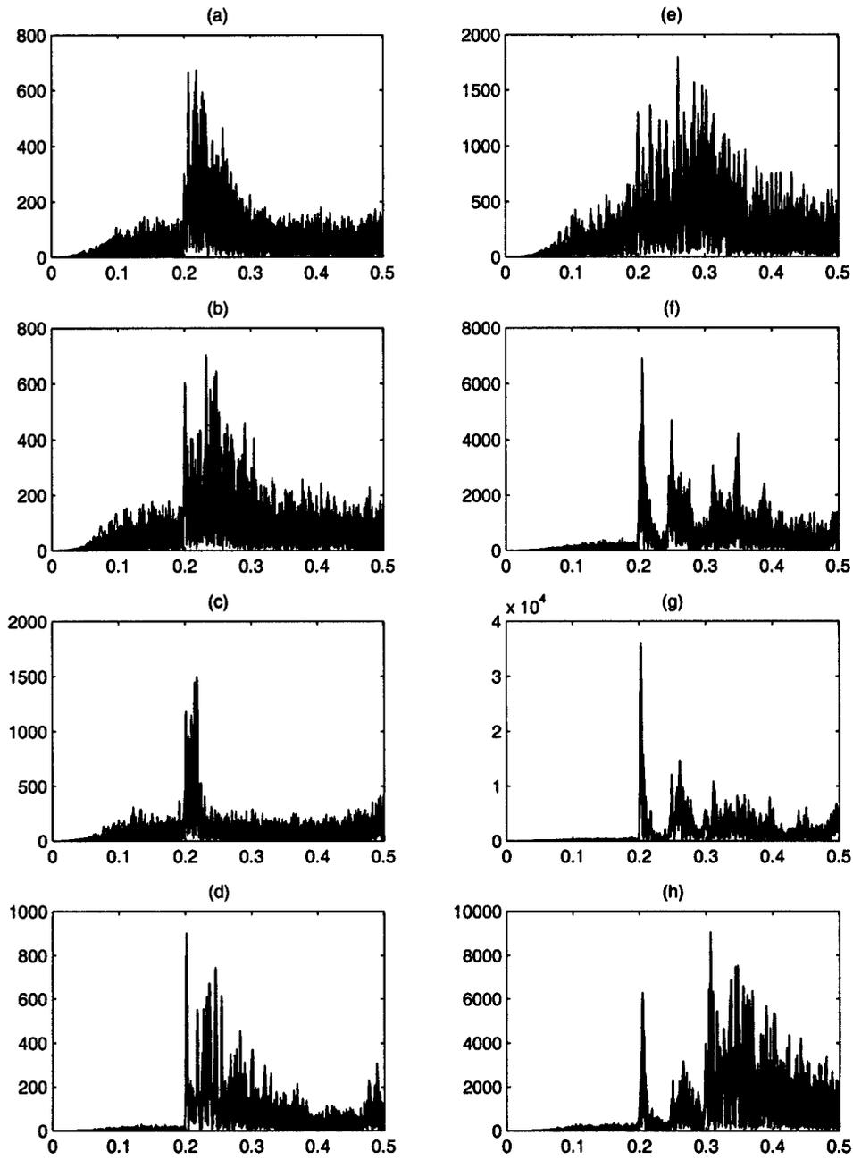
Figure 4.7 - NBOA98 Deep (a-d) and Shallow (e-h) Water Channel Responses
