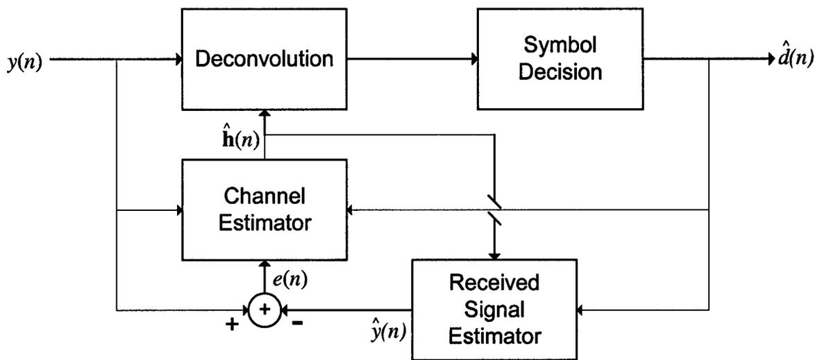
**Figure 4.10 - Block Diagram of the EQSID Method in Decision Directed Mode**
