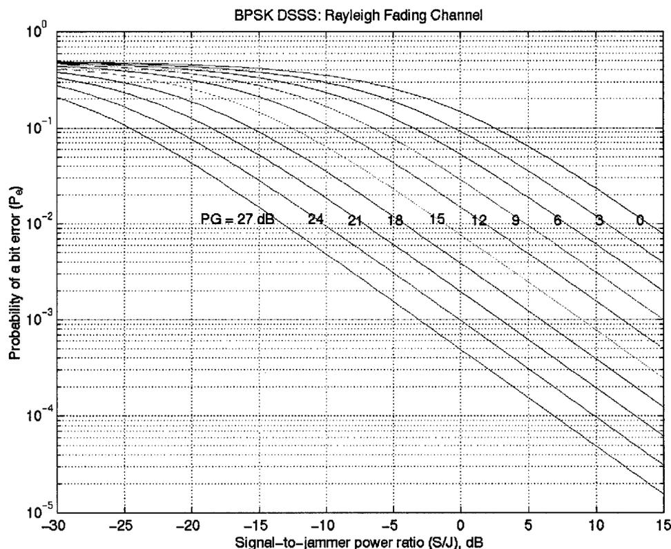
**Figure 4.13 - BPSK DSSS Performance in a Rayleigh-Fading Channel**
