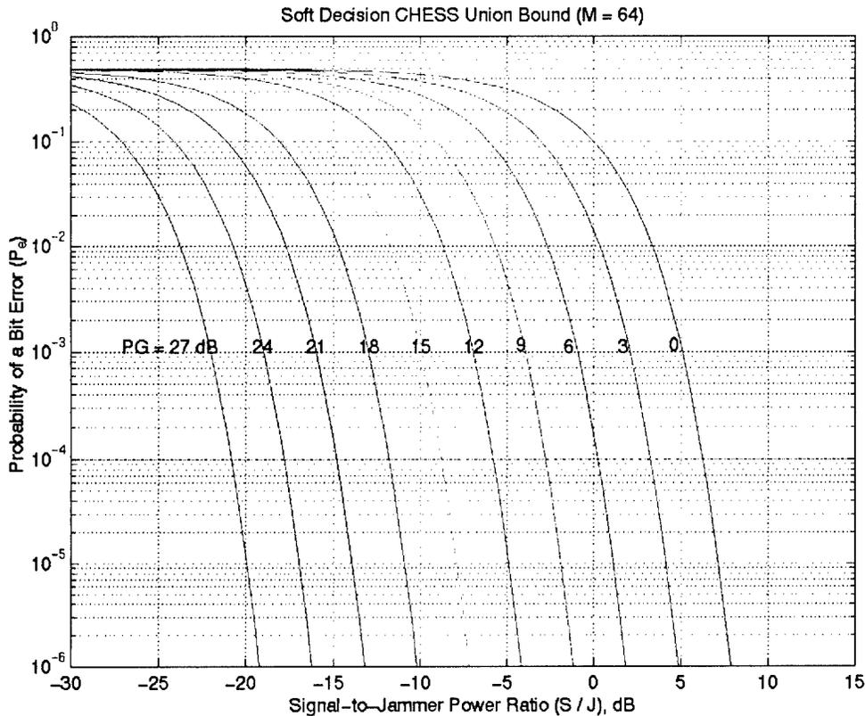
**Figure 4.14 - Acoustic CHES Performance in an AWGN Channel**
