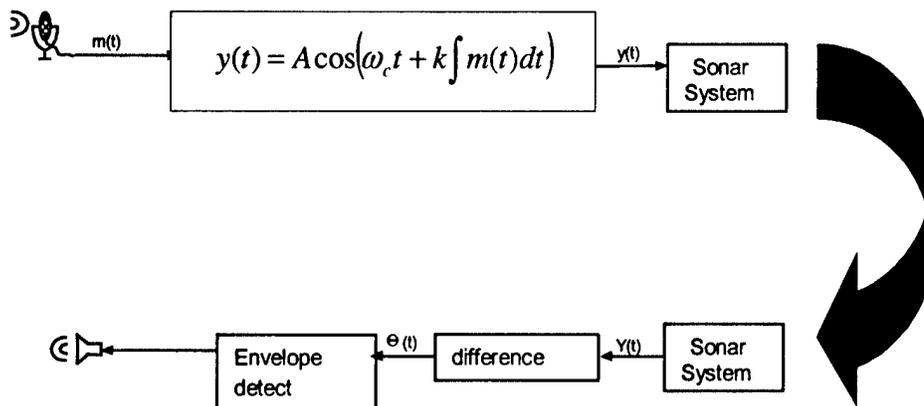
**Figure 4.2 - Block Diagram of Frequency Modulated System**
