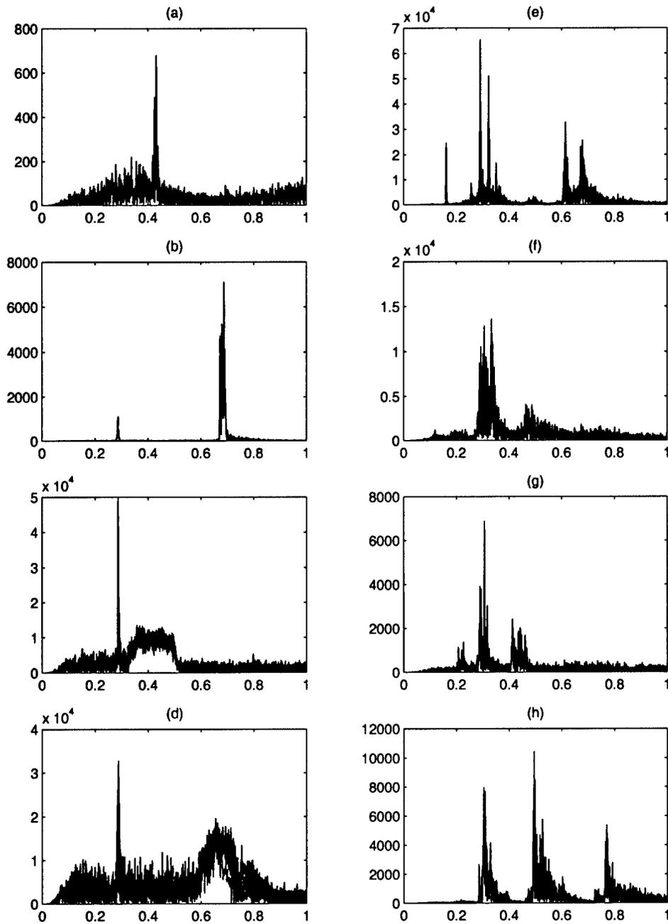
**Figure 4.8 - FBE Echo Deep (a-d) and Shallow (e-h) Water Channel Responses**
