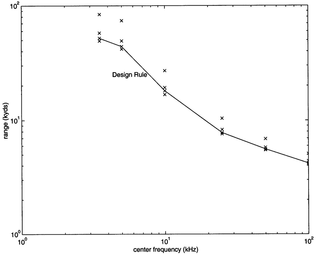
Figure 7.5 - Rules-of-Thumb, Range vs. Center frequency
