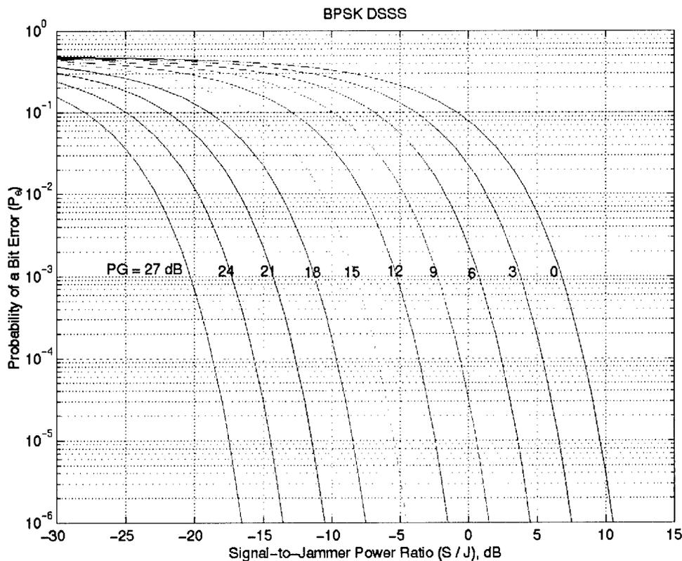
Figure 4.12 - BPSK DSSS Performance in an AWGN Channel
