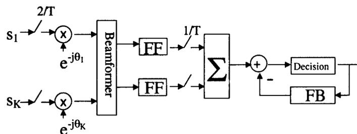
Figure 4.4 - Multichannel Decision Feedback Equalizer
