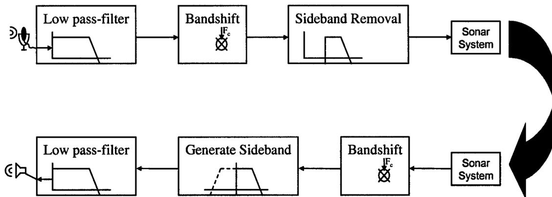
**Figure 4.1 - Block Diagram of Single-Side-Band Amplitude Modulation**
