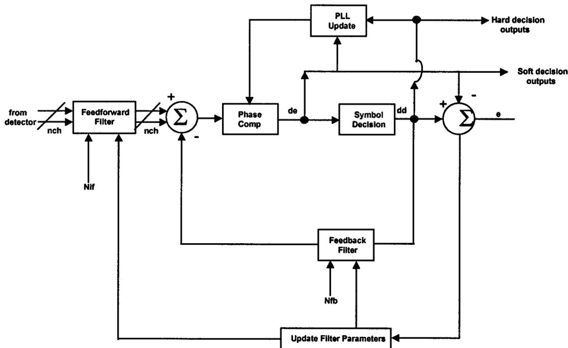
Figure 4.3 - Decision Feedback Equalizer Block Diagram
