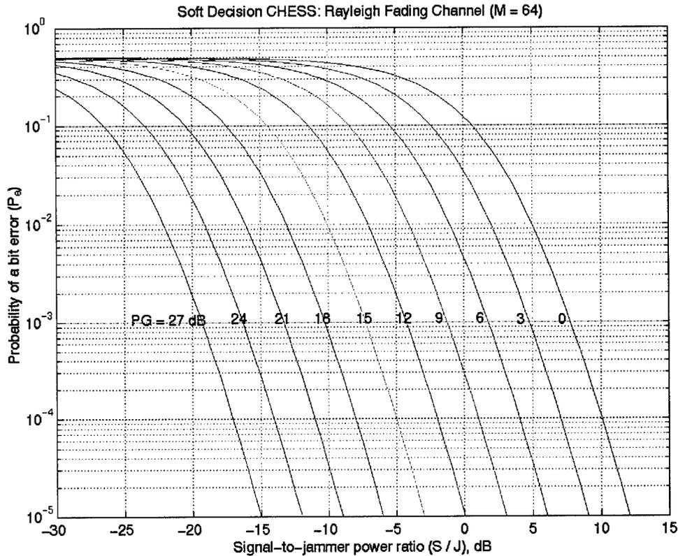
Figure 4.15 - Acoustic CHES Performance in a Rayleigh-Fading Channel
