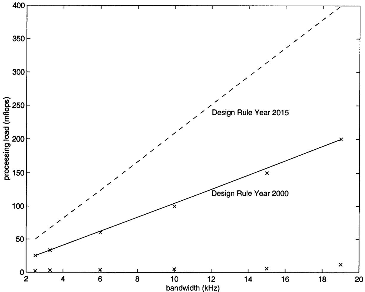
Figure 7.6 - Rules-of-Thumb, Processing Load vs. Bandwidth
