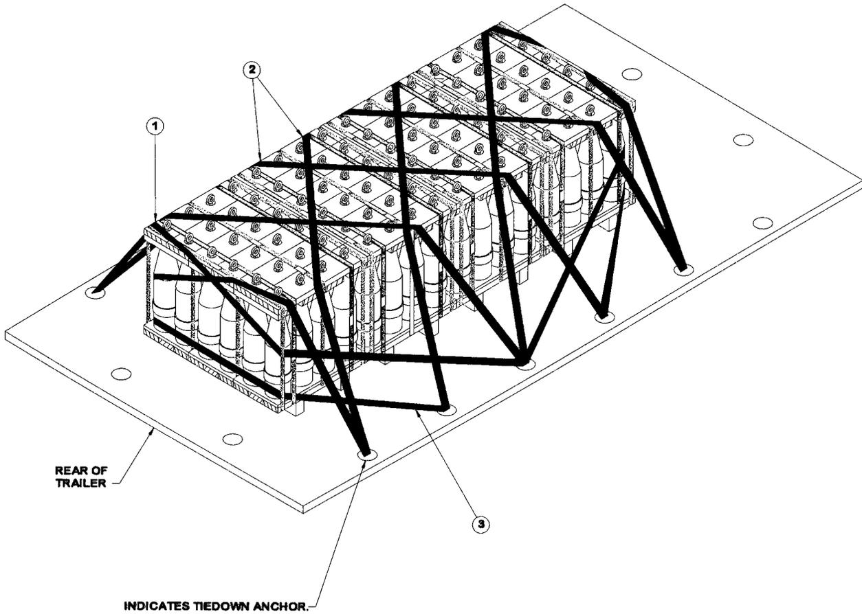
NOTE: THIS DRAWING SHOWS STRAP ASSEMBLIES AT IMPROVED LOCATIONS DETERMINED BY TESTING.
