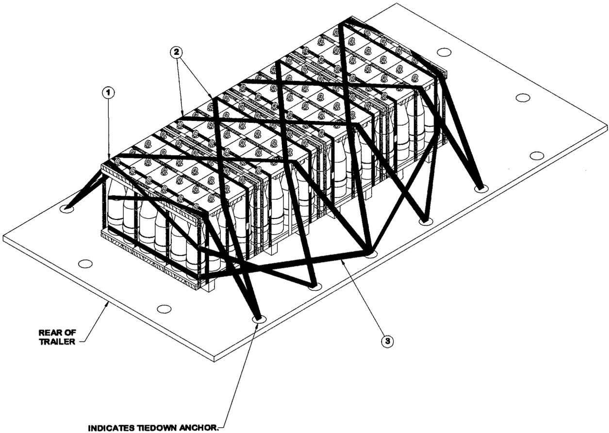
**NOTE: THIS DRAWING SHOWS STRAP ASSEMBLIES AS TESTED.
