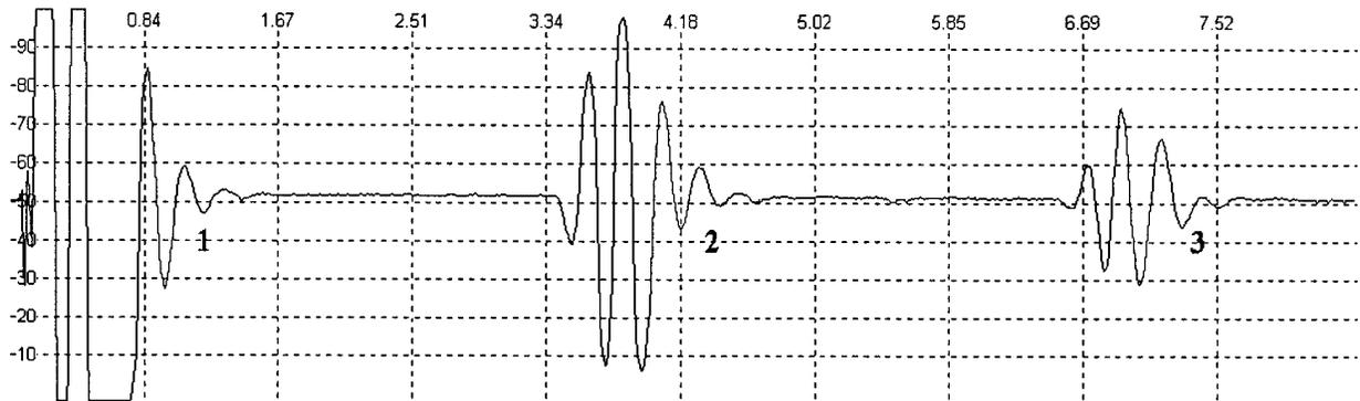
**Figure 3. Ultrasonic Wave Train From a Ti-6Al-4V Specimen.**
