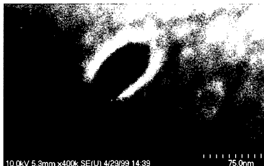
Fig. 4. Field emission scanning electron micrograph of solid solution in a 50 nm wide via in \text{Si}_3\text{N}_4 on an underlying silver electrode.
